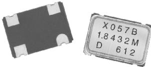
The XOSM-573 series is an ultra miniature package clock oscillator with dimensions 7.0 x 5.0 x 1.6 mm. It is mainly used in portable PC and telecommunication devices and equipment.
