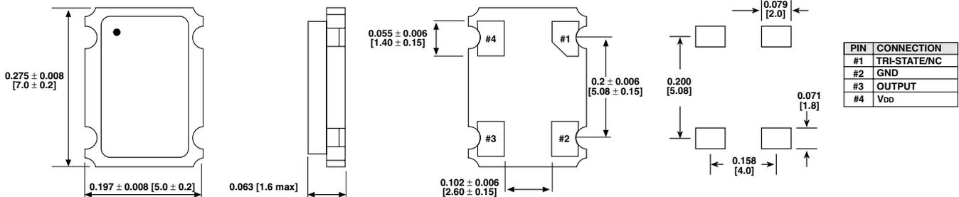
\*\*\*note: A 0.01 μF bypass capacitor should be placed between VDD(Pin4) and GND(Pin2) to minimize power supply line noise
