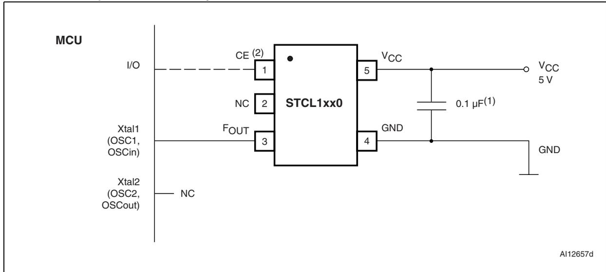
1. For reliable operation and to further improve immunity to harsh environment, the minimum 0.1 µF decoupling capacitor is recommended to be placed as close as possible to the V<sub>CC</sub> and GND pins of the oscillator device. The whole oscillator block should then be placed near the microprocessor clock input.
