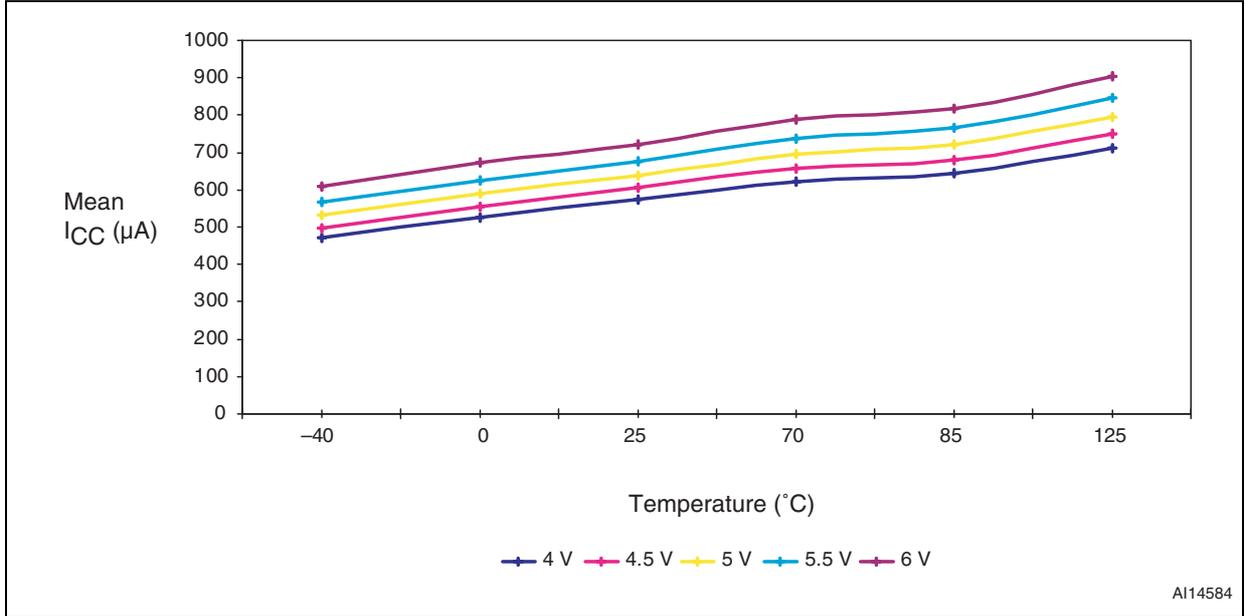
Figure 6. Standby supply current vs. temperature, STCL1120
