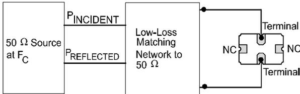
$$\text{CW RF Power Dissipation} = P_{\text{INCIDENT}} - P_{\text{REFLECTED}}$$
