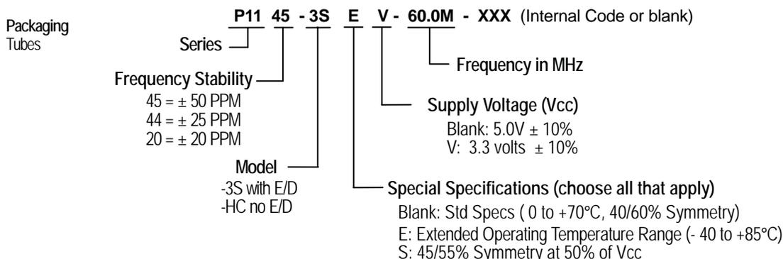
Consult factory for available frequencies and specs. Not all options available for all frequencies. A special part number may be assigned. Frequency Stability is inclusive of frequency shifts due to calibration, temperature, supply voltage, shock, vibration and load
