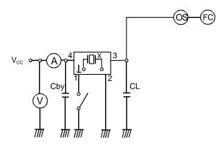
CL; 15pF MAX including input capacity of osilloscope
