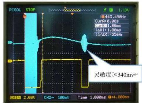
4) Decay Time Test: 40K-Test Jig connected with Oscilloscope (OSC),
