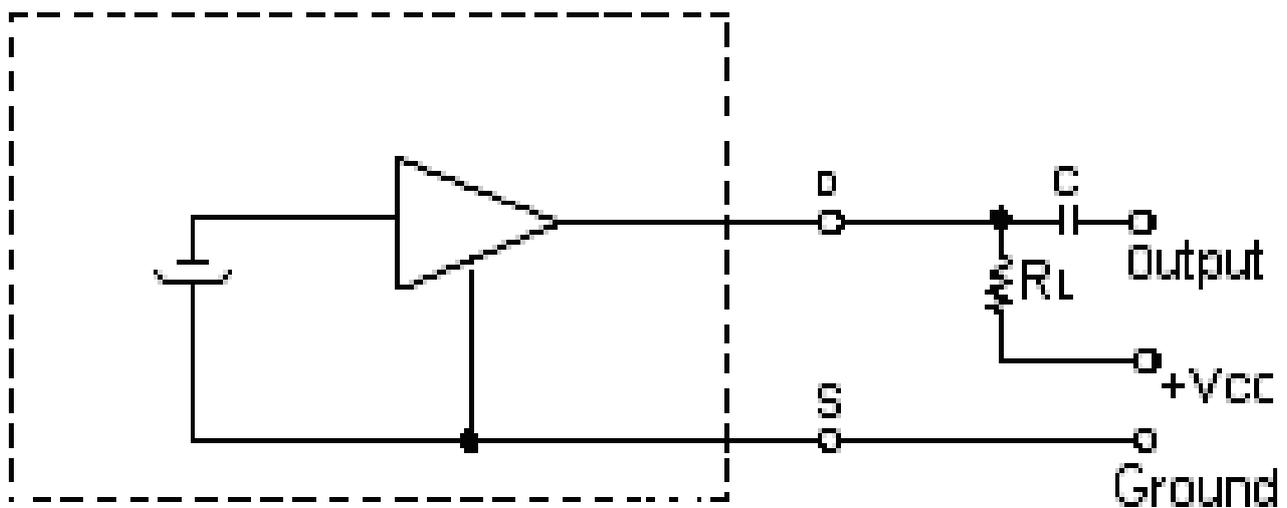
$R_L=2.2k\ \Omega$  (External resistor)       $+V_{CC}=4.5V$        $C=1\mu F$
