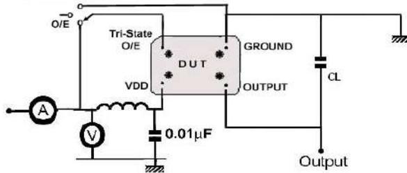
Output to oscilloscope and/or frequency counter
