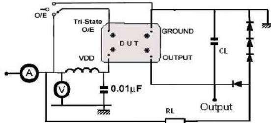
Output to oscilloscope and/or frequency counter
