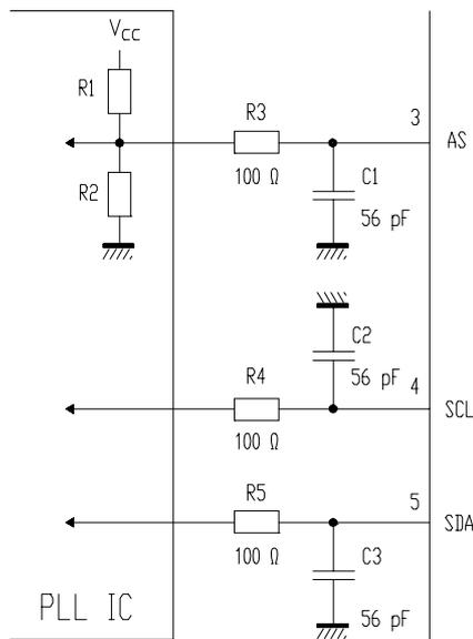
Fig.4 I<sup>2</sup>C-bus load.
