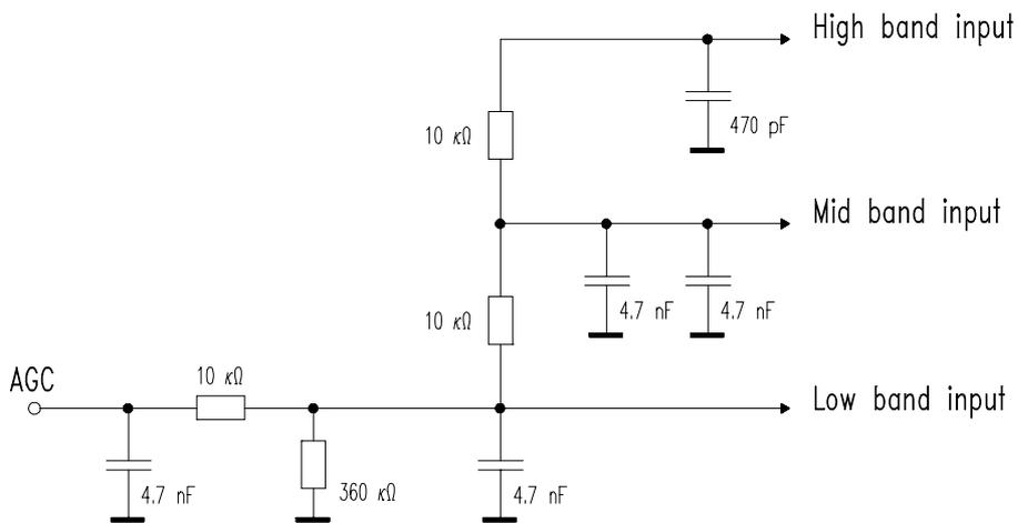
Fig.5 Internal AGC circuit.
