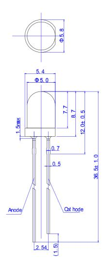
All dimensions in mm, tolerances unless mentioned is ±0.2 mm.
