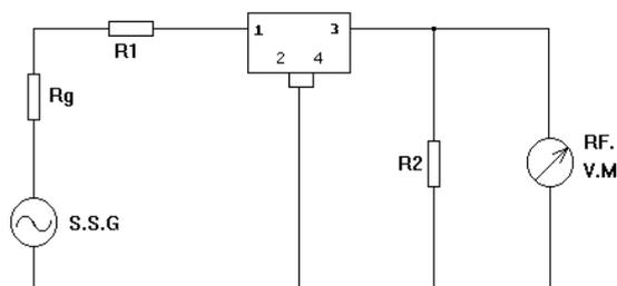
$R_g + R_1 = R_2 = \text{Input/Output Impedance}$
