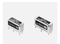
The following lines of filters are high performance devices that achieve ultimate stopband attenuation through the use of multiple piezoelectric elements connected in ladder form. A few of the recommended applications for these filters include high class receivers, SSB communications equipment, pocket pagers and mobile radios.
