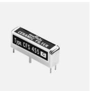
The following lines of filters are high performance devices that achieve ultimate stopband attenuation through the use of multiple piezoelectric elements connected in ladder form. A few of the recommended applications for these filters include high class receivers, SSB communications equipment, pocket pagers and mobile radios.
