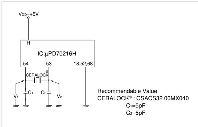
Application to CXD2510Q (SONY) (Digital Signal Processing IC for CD)
