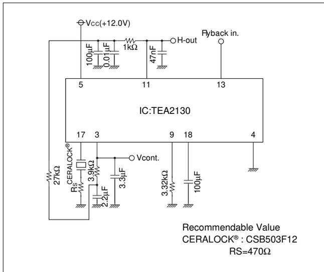
**Oscillation Circuit incorporating Transistor**
