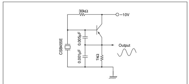
**Application to MC13022P (MOTOROLA) (AM Stereo Decoder)**
