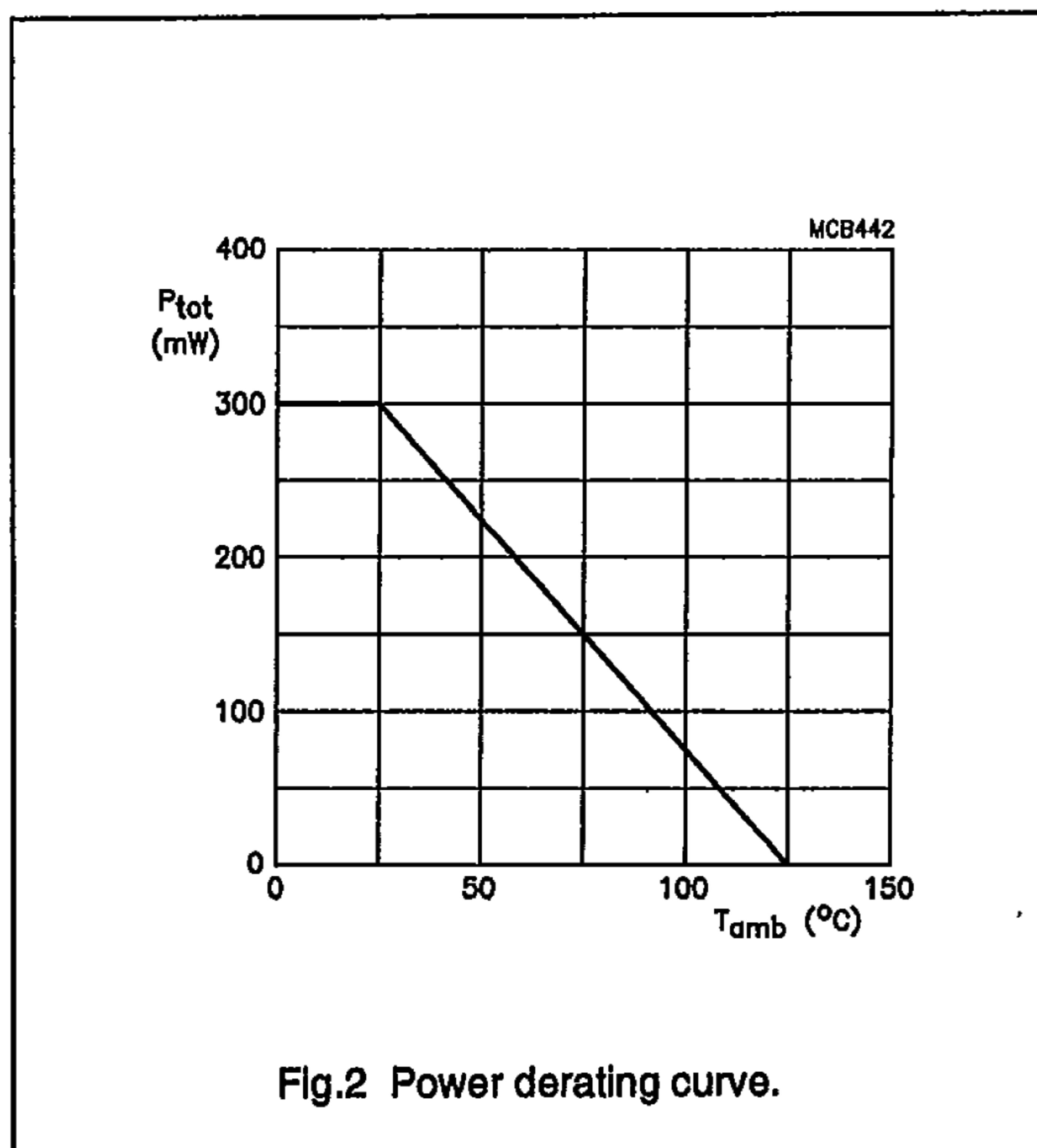
Fig.2 Power derating curve.
