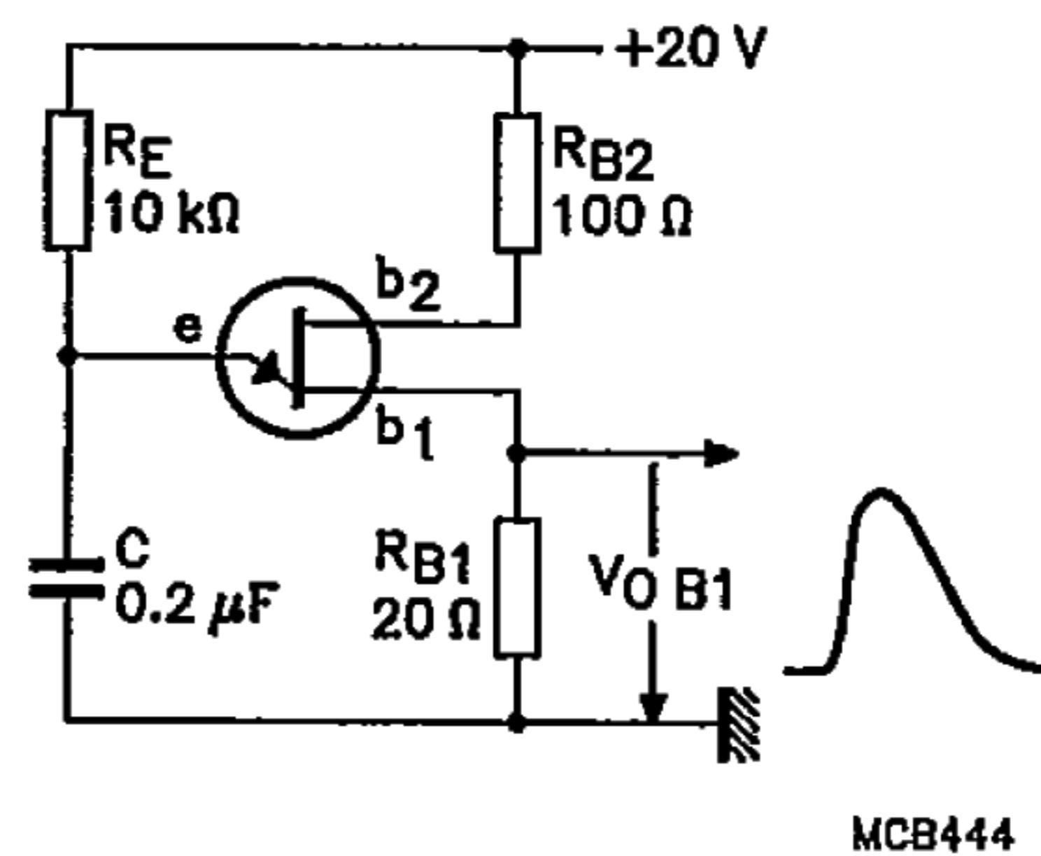
Fig.4 Impulse output circuit.
