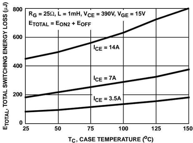
FIGURE 15. TOTAL SWITCHING LOSS vs CASE TEMPERATURE
