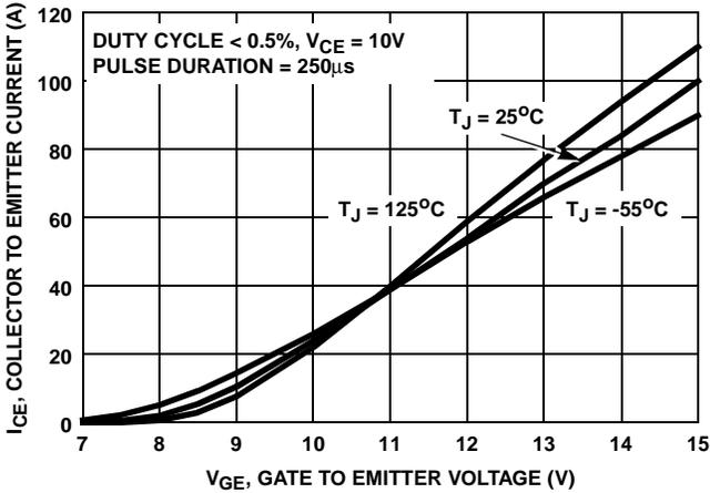
FIGURE 13. TRANSFER CHARACTERISTIC
