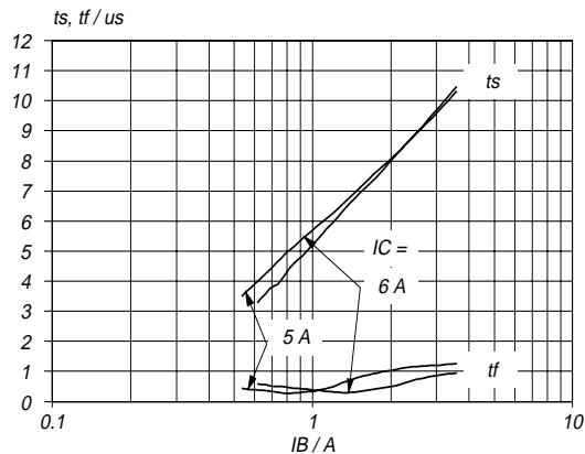
Fig.10. Typical collector storage and fall time.
