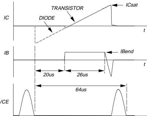
Fig. 1. Switching times waveforms (16 kHz).
