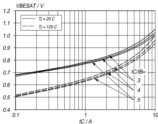
Fig. 5. Typical base-emitter saturation voltage.  $V_{BE\text{sat}} = f (I_C)$ ; parameter  $I_C/I_B$
