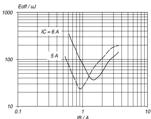
Fig.9. Typical turn-off losses.  $T_j = 85^\circ\text{C}$
