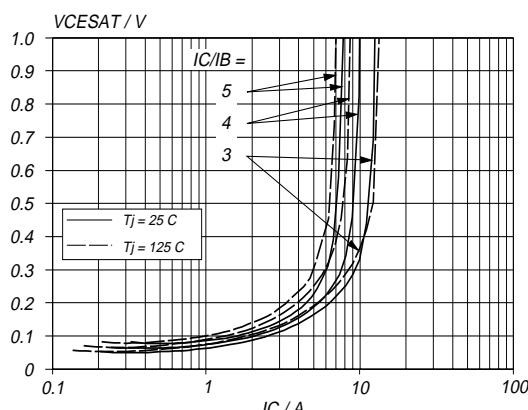
Fig. 6. Typical collector-emitter saturation voltage.  $V_{CE\text{sat}} = f (I_C)$ ; parameter  $I_C/I_B$
