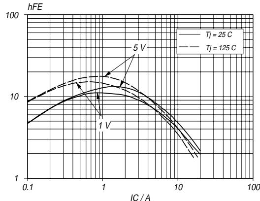
Fig. 4. Typical DC current gain.  $h_{FE} = f (I_C)$  parameter  $V_{CE}$
