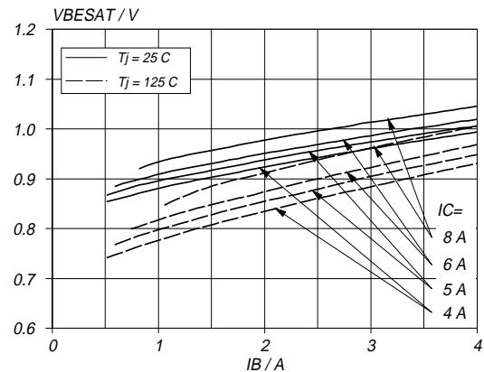
Fig.7. Typical base-emitter saturation voltage.
