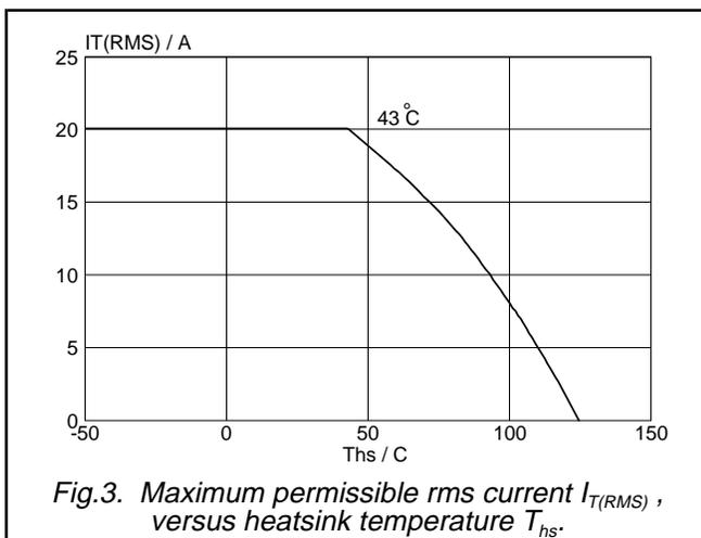
Fig. 3. Maximum permissible rms current  $I_{T(RMS)}$ , versus heatsink temperature  $T_{hs}$ .
