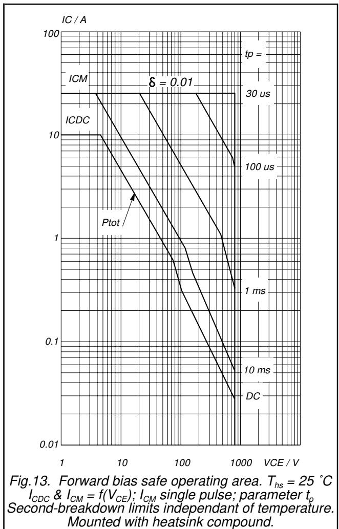
Fig.13. Forward bias safe operating area.  $T_{hs} = 25^\circ\text{C}$
