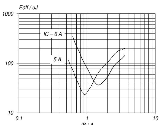
Fig.9. Typical turn-off losses.  $T_j = 85^\circ C$
