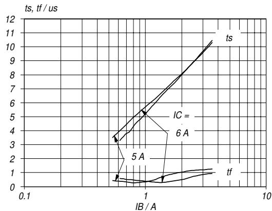
Fig.10. Typical collector storage and fall time.
