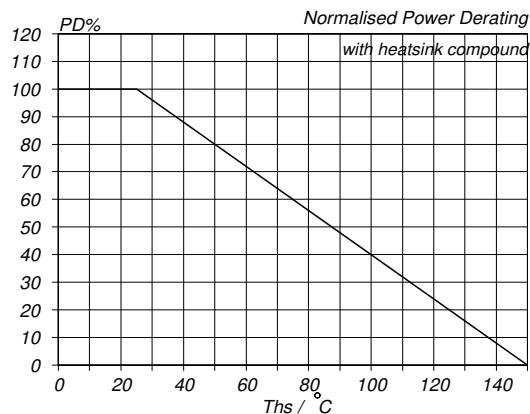
Fig.11. Normalised power dissipation.
