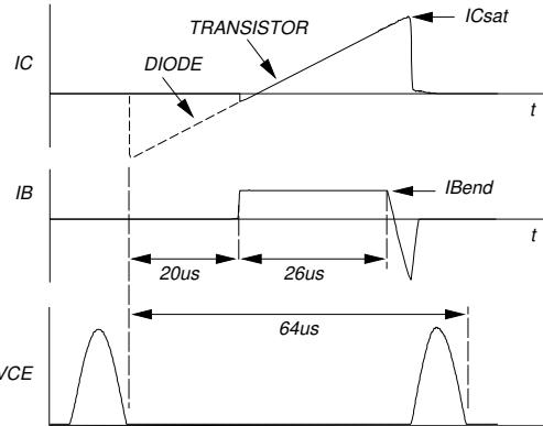
Fig. 1. Switching times waveforms (16 kHz).
