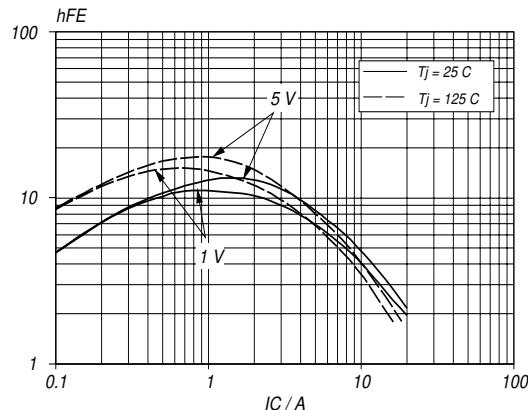
Fig. 4. Typical DC current gain.  $h_{FE} = f (I_C)$  parameter  $V_{CE}$
