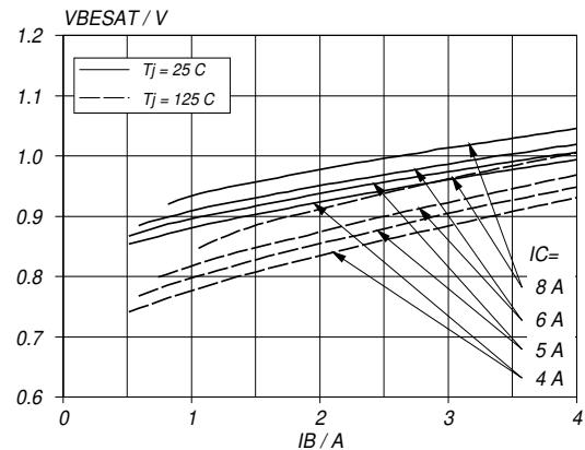
Fig.7. Typical base-emitter saturation voltage.
