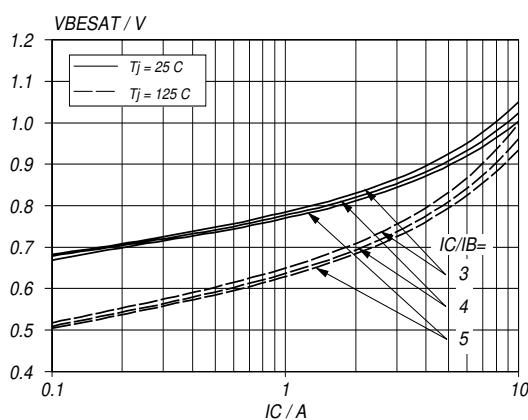
Fig. 5. Typical base-emitter saturation voltage.  $V_{BEsat} = f (I_C)$ ; parameter  $I_C/I_B$
