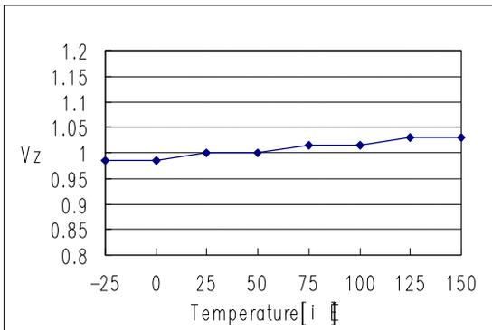
**Figure 9. V<sub>CC</sub> Zener Voltage**
