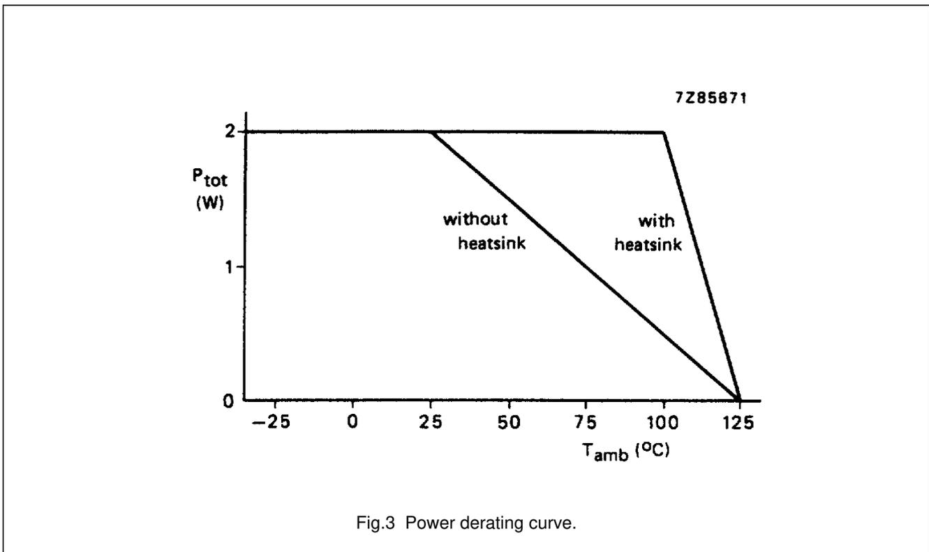
Fig.3 Power derating curve.
