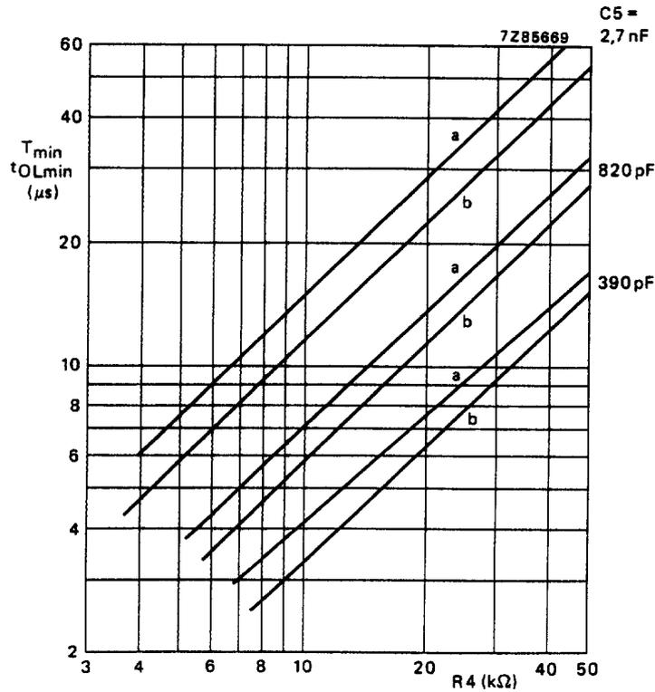
Fig.6 Minimum output pulse repetition time  $T_{min}$  (curves a) and minimum output LOW time  $t_{OLmin}$  (curves b) in the frequency regulation mode as a function of external resistor  $R4$  connected between RX and ground with external capacitor  $C5$  connected between CX and ground as a parameter.
