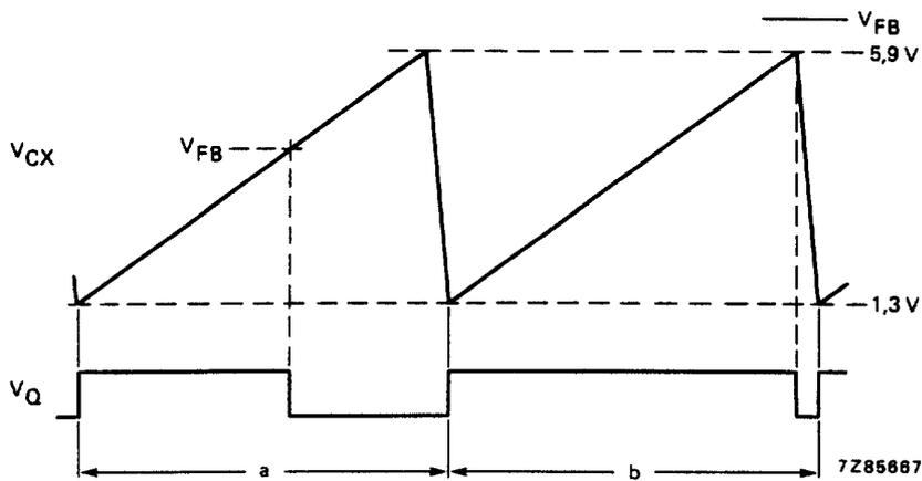
Fig.7 Timing diagram for the duty factor regulation mode showing the voltage on external capacitor  $C5$  connected between CX and ground and the output voltage as a function of time for two combinations of input signals. *a*: The voltages on inputs FB or LIM are below 5,9 V. The circuit is in its normal regulation range. *b*: The voltages on inputs FB and LIM are higher than 5,9 V. The circuit produces its minimum output LOW time, giving the maximum duty factor of the SMPS.
