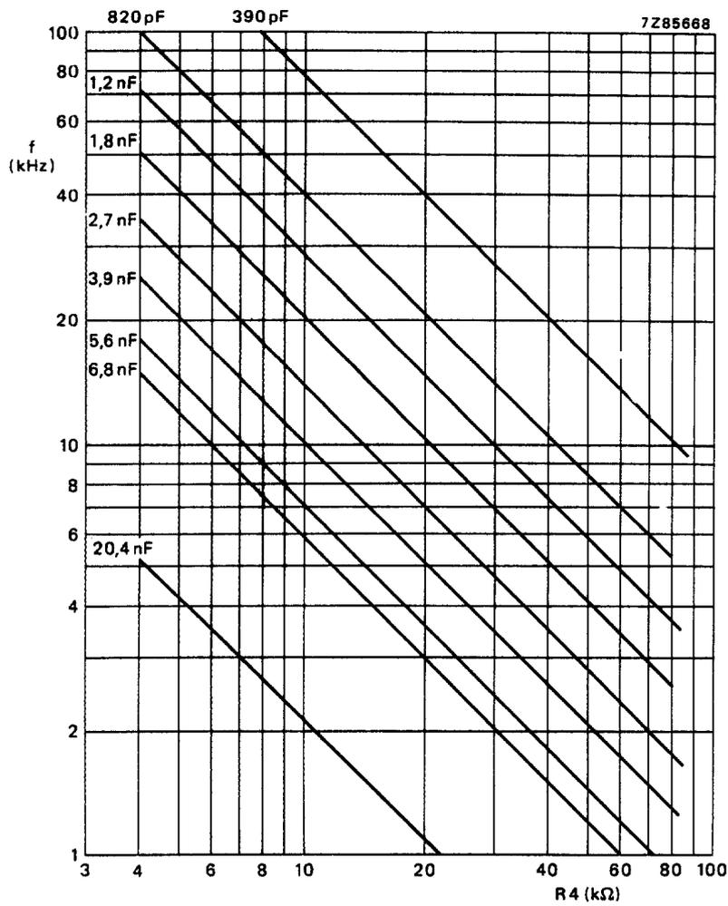
Fig.4 Minimum pulse repetition frequency in the frequency regulation mode, and working pulse repetition frequency in the duty factor regulation mode, as a function of external resistor R4 connected between RX and ground with external capacitor C5 connected between CX and ground as a parameter.
