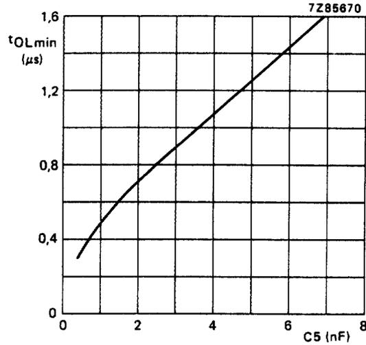
Fig.8 Minimum output LOW time  $t_{OLmin}$  in the duty factor regulation mode as a function of external capacitor  $C5$  connected between CX and ground. In this mode the minimum output LOW time is independent of  $R4$  for values of  $R4$  between 4 k $\Omega$  and 80 k $\Omega$ .
