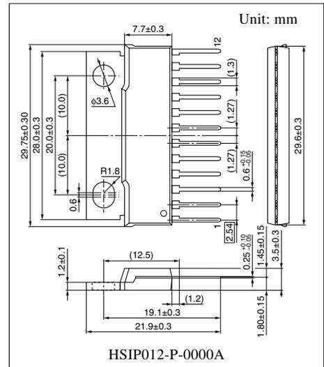
Note) The package of this product will be changed to lead-free type (HSIP012-P-0000E). See the new package dimensions section later of this datasheet.
