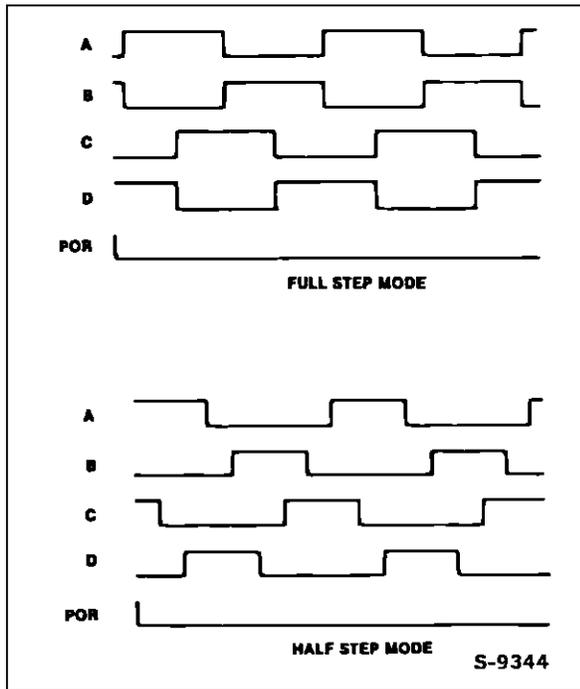
When implementing a half step drive, both outputs of the L6506 will be low during the half step of one phase. This means a very long time is required for the current in the "off" winding to decay when driving bipolar motors.
