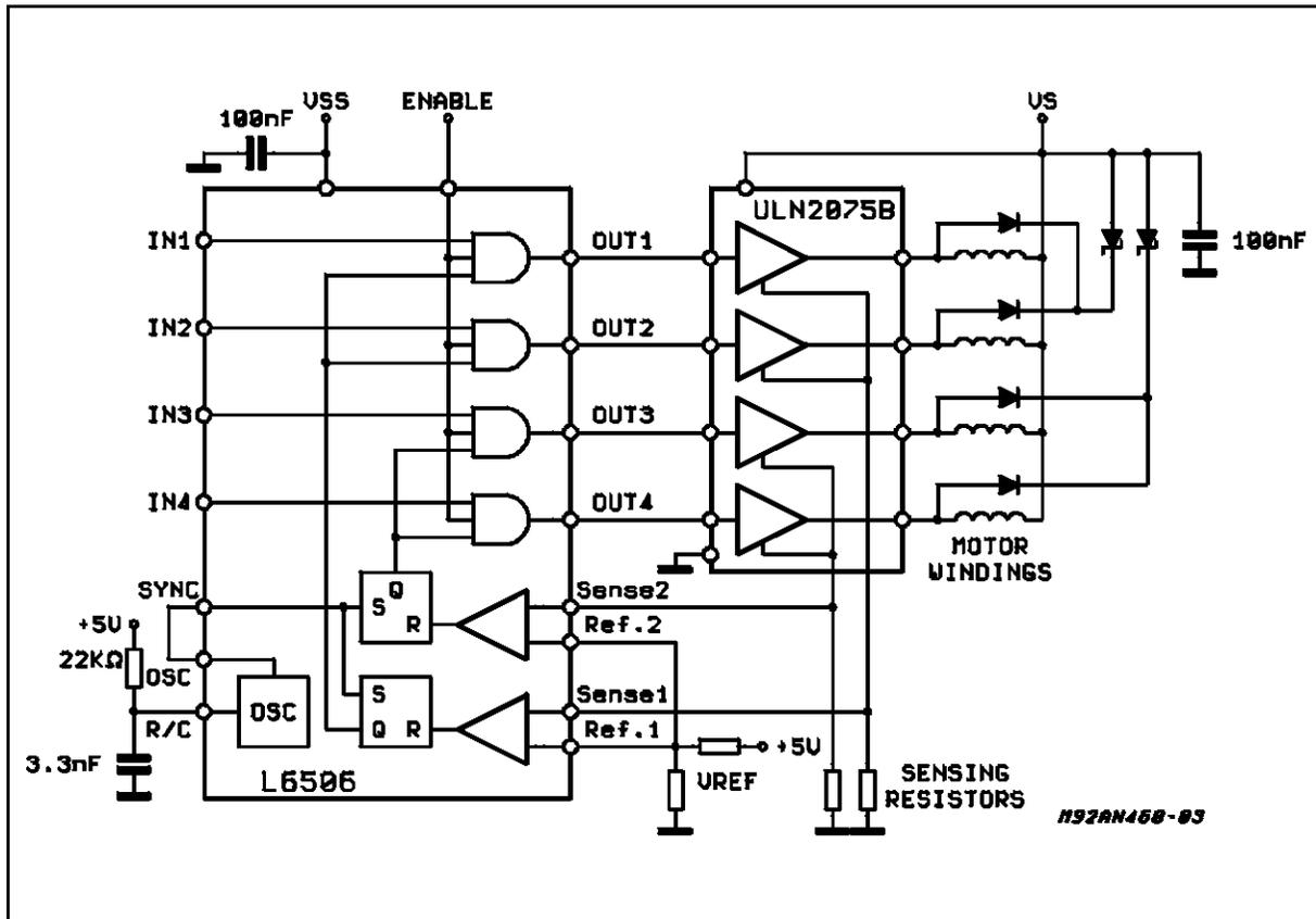
When the current in the load winding reaches the programmed peak value, the voltage across the sense resistor ( $R_{sense}$ ) is equal to reference voltage input ( $V_{ref}$ ) and the corresponding comparator resets its flip-flop. This interrupts the drive and allows the current to decay through a recirculating path until the next oscillator pulse occurs. The peak current in each winding is programmed by selecting the value of the sense resistor and  $V_{ref}$  and is given by the equation :
