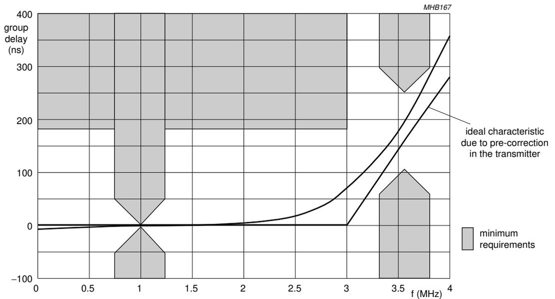
Overall delay is not shown, here the maximum ripple is specified.
