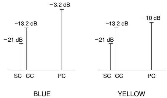
SC is sound carrier, with respect to sync level.
