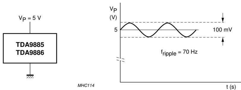
Fig.6 Ripple rejection condition.
