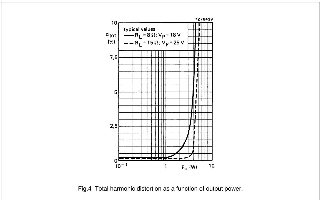
Fig.4 Total harmonic distortion as a function of output power.
