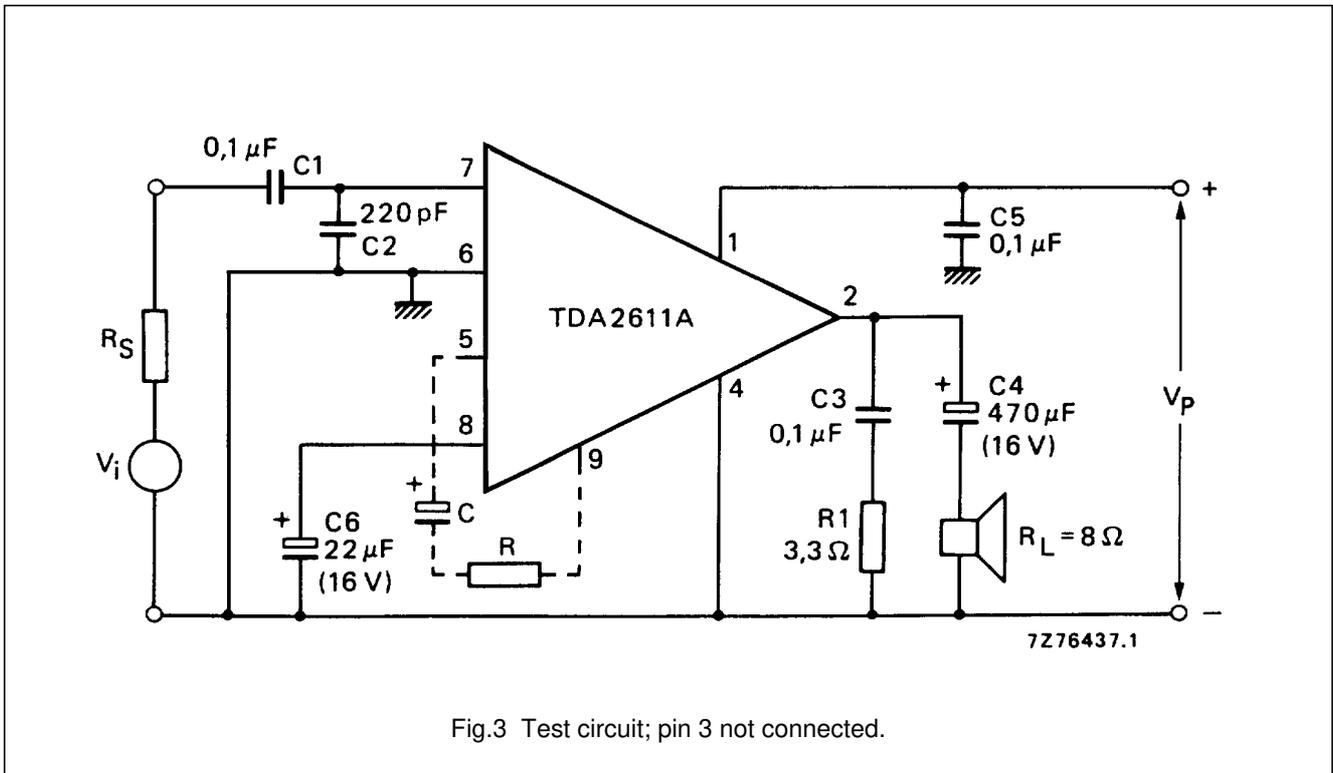
Fig.3 Test circuit; pin 3 not connected.
