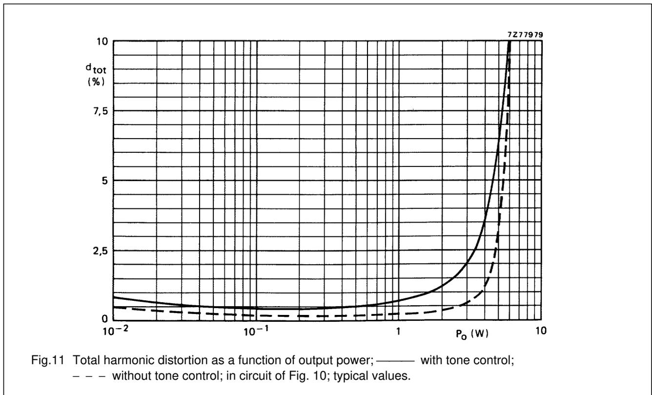
Fig.11 Total harmonic distortion as a function of output power; — with tone control; - - - without tone control; in circuit of Fig. 10; typical values.
