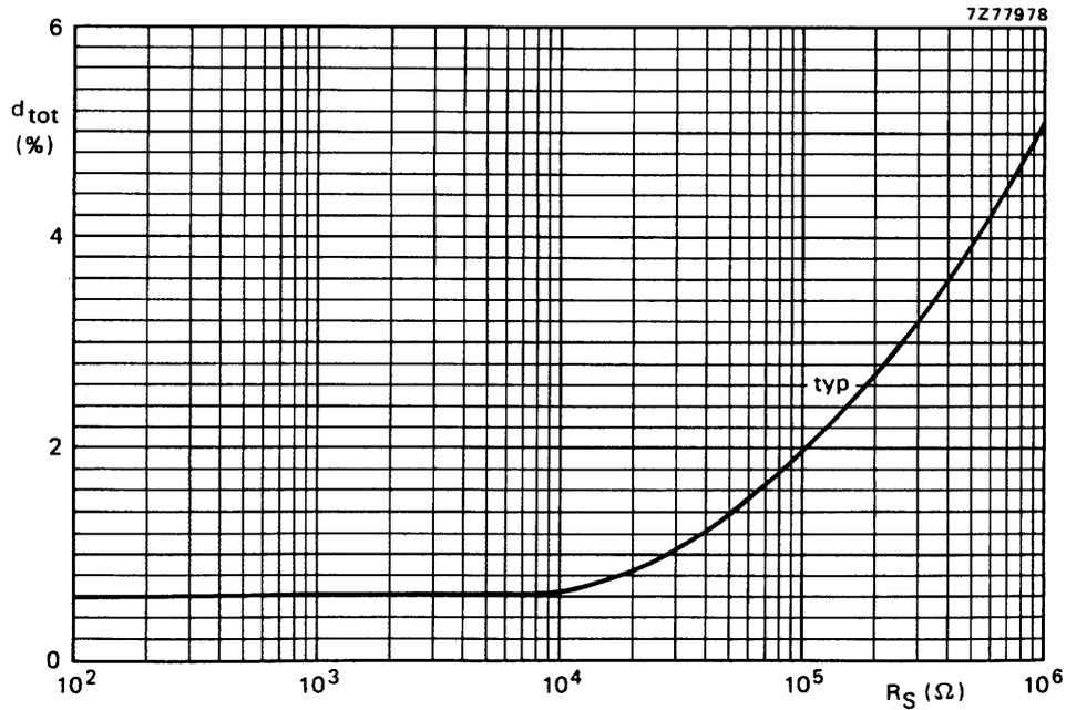
Fig.8 Total harmonic distortion as a function of R<sub>S</sub> in the circuit of Fig. 3; P<sub>o</sub> = 3,5 W; f = 1 kHz.
