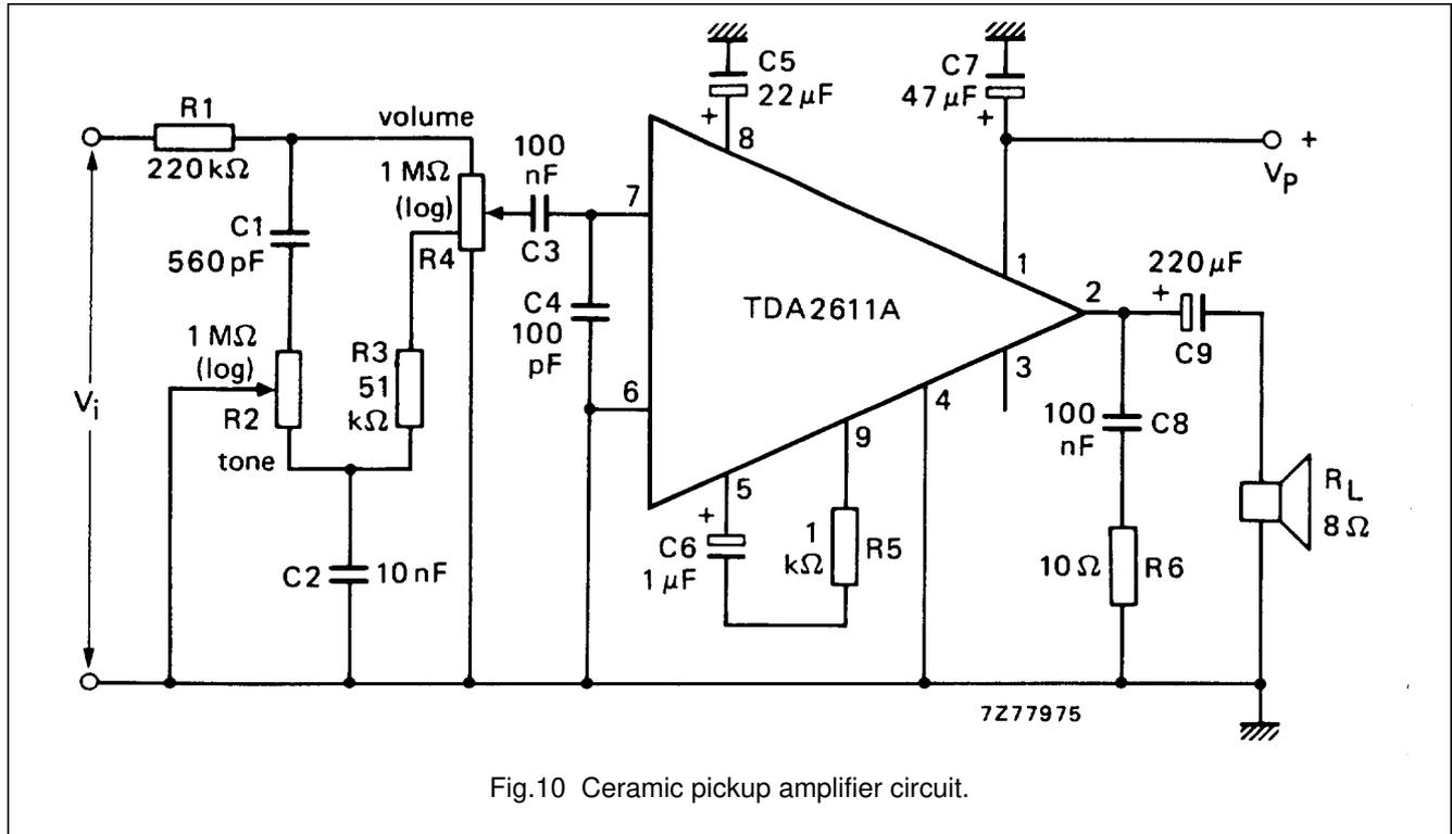
Fig.10 Ceramic pickup amplifier circuit.
