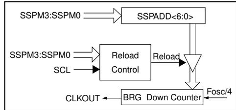
**FIGURE 15-22: BAUD RATE GENERATOR TIMING WITH CLOCK ARBITRATION**
