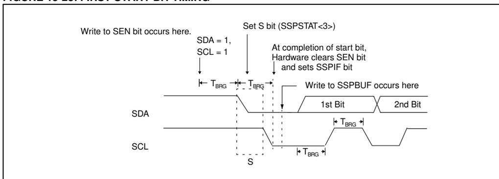
**FIGURE 15-24: START CONDITION FLOWCHART**
