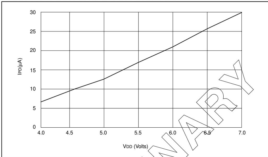
**FIGURE 21-12: MAXIMUM  $I_{PD}$  vs.  $V_{DD}$  WATCHDOG ENABLED**
