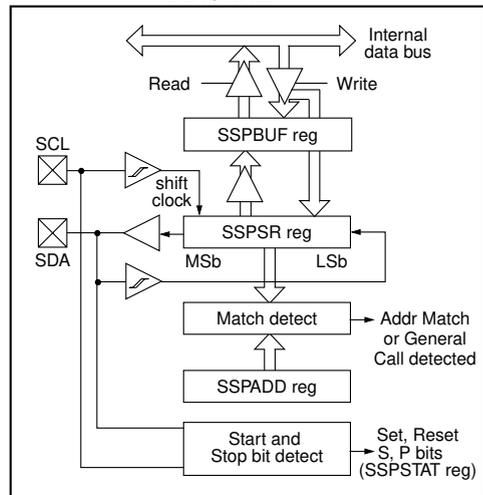
**FIGURE 15-3: I<sup>2</sup>C MASTER MODE BLOCK DIAGRAM**
