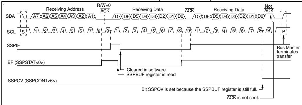
**FIGURE 15-16: I<sup>2</sup>C WAVEFORMS FOR TRANSMISSION (7-BIT ADDRESS)**
