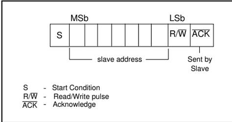
FIGURE E-3: I<sup>2</sup>C 10-BIT ADDRESS FORMAT
