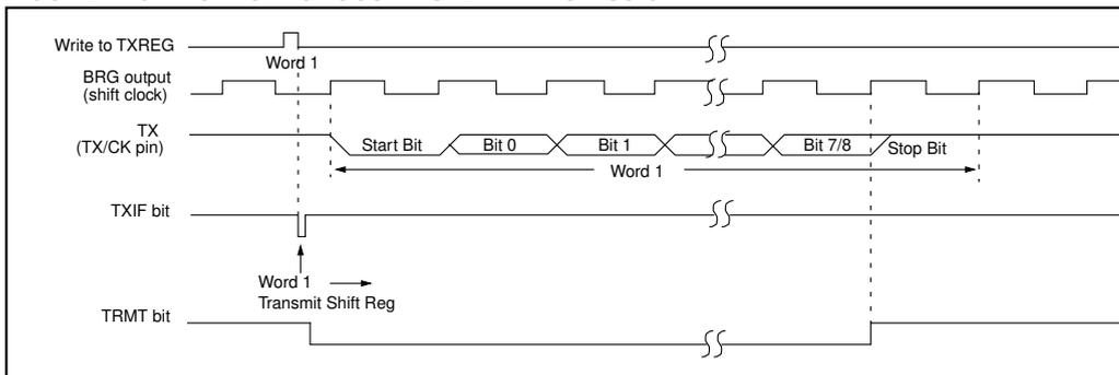
**FIGURE 14-6: ASYNCHRONOUS MASTER TRANSMISSION (BACK TO BACK)**
