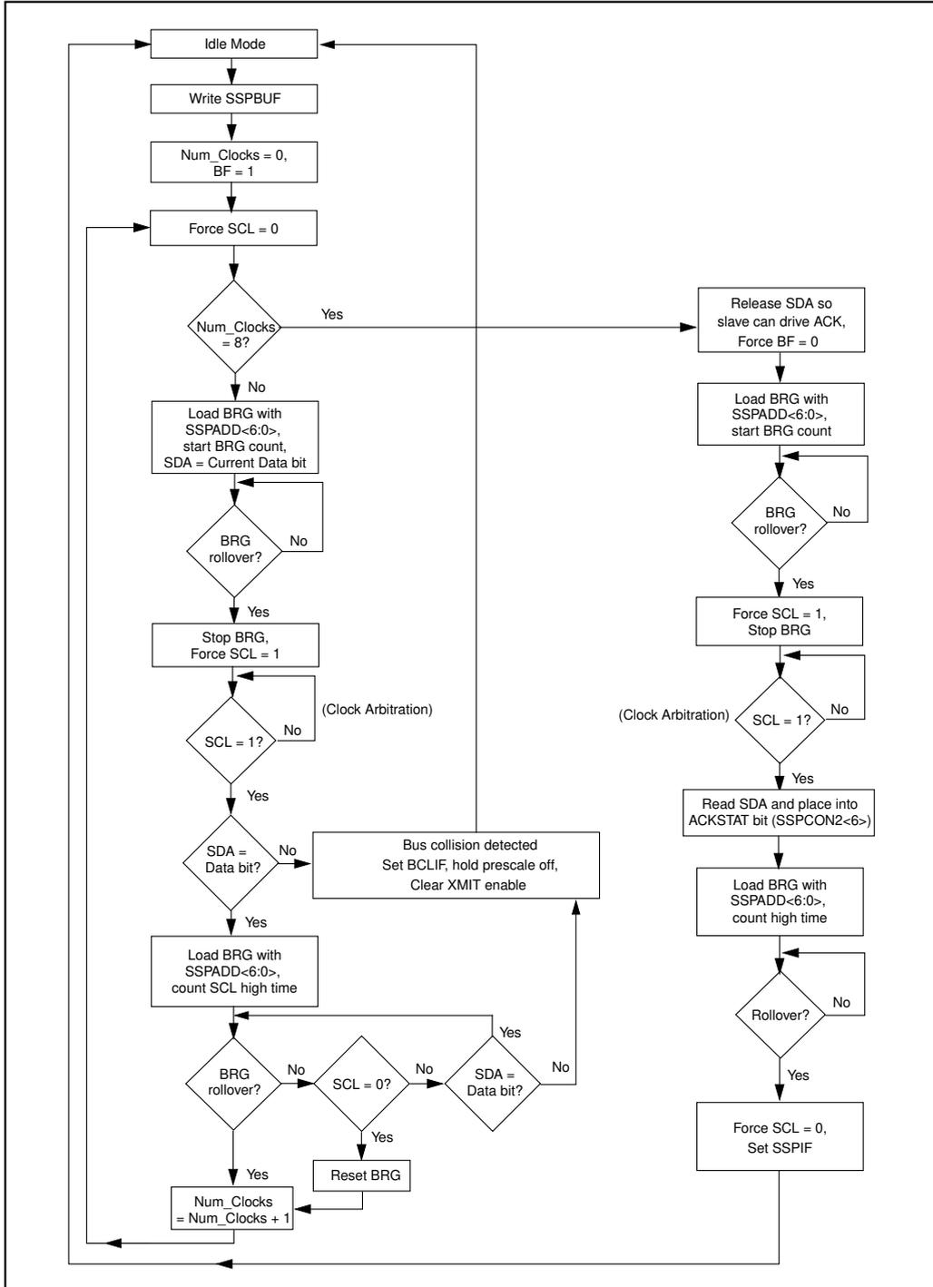
**FIGURE 15-29: I<sup>2</sup>C MASTER MODE TIMING (TRANSMISSION, 7 OR 10-BIT ADDRESS)**
