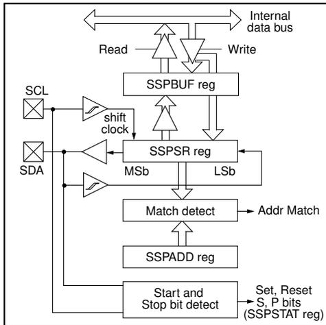
**FIGURE 15-14: I<sup>2</sup>C MASTER MODE BLOCK DIAGRAM**
