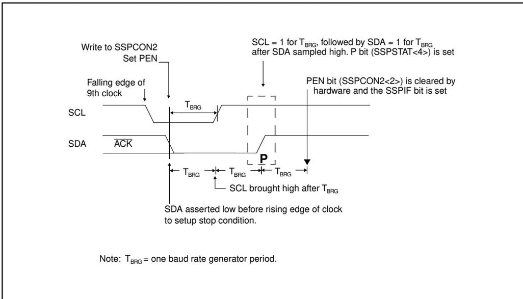
**FIGURE 15-35: STOP CONDITION FLOWCHART**
