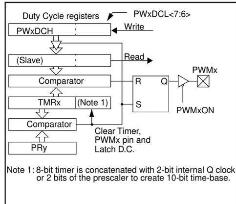
**FIGURE 13-7: PWM OUTPUT (NOT BUFFERED)**
