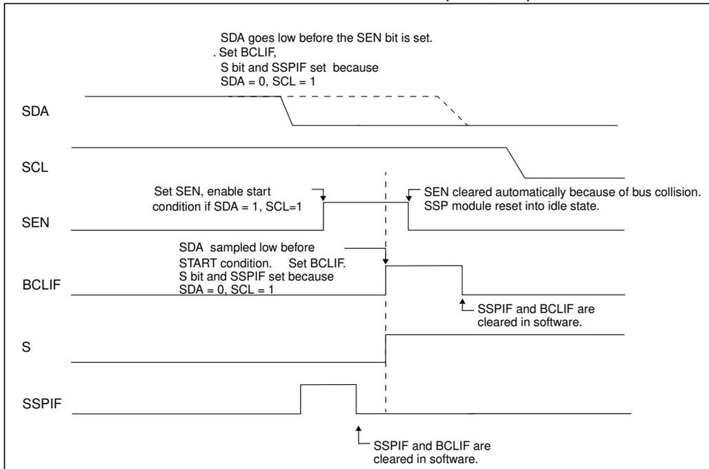
**FIGURE 15-39: BUS COLLISION DURING START CONDITION (SCL = 0)**
