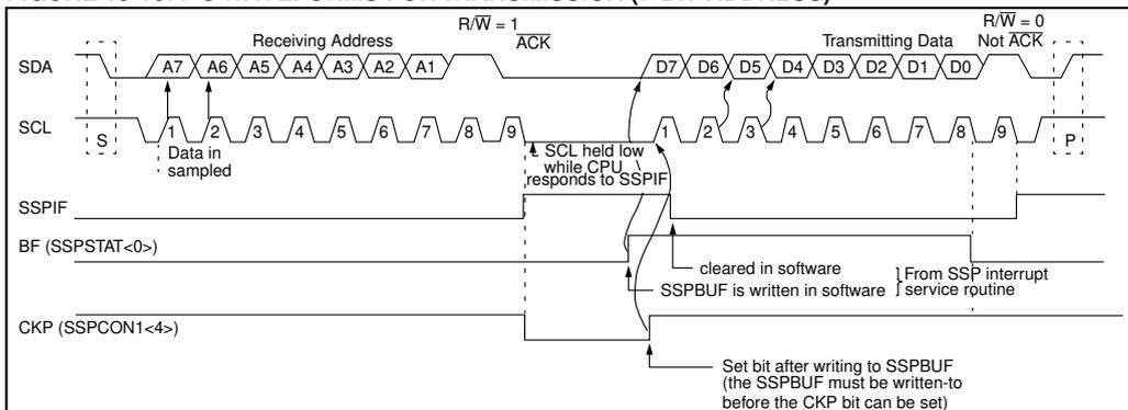
**FIGURE 15-17: I<sup>2</sup>C SLAVE-TRANSMITTER (10-BIT ADDRESS)**
