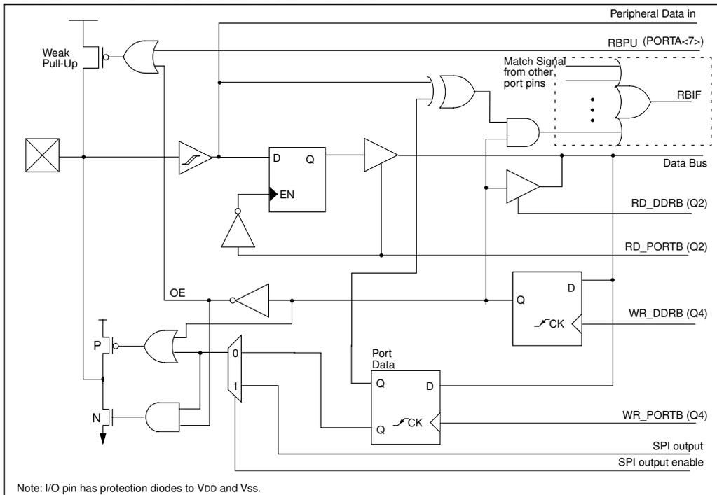
**FIGURE 10-8: BLOCK DIAGRAM OF RB7 PORT PIN**
