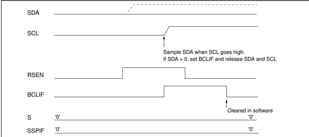
**FIGURE 15-42: BUS COLLISION DURING REPEATED START CONDITION (CASE 2)**
