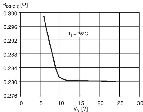
**Figure 6. Typical High-Side  $R_{DS(ON)}$  vs. Supply Voltage**
