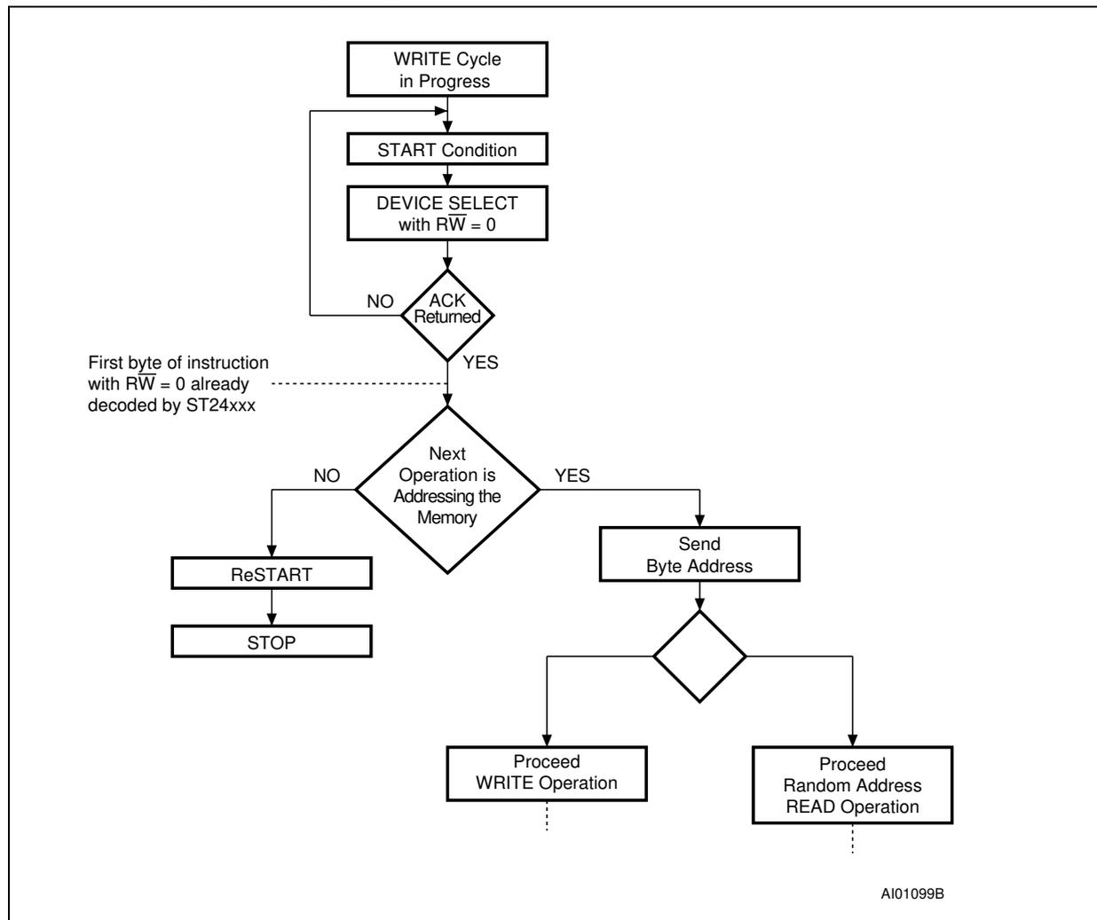
Figure 8. Write Modes Sequence (ST24/25C02 and ST24C02R)
