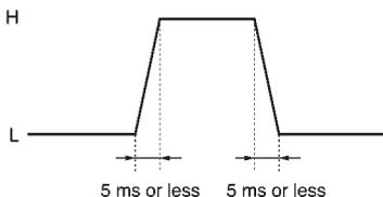
Fig.17 Control signal
