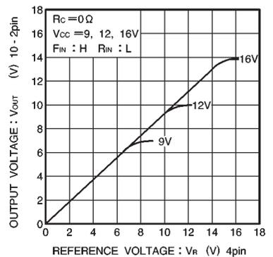
Fig.12 Output voltage vs. reference voltage ( I )
