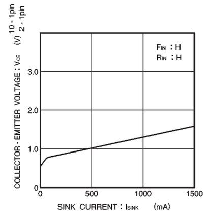
Fig.9 Output saturated voltage vs. sink current ( II )
