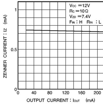
Fig.14 Zener current vs. output current
