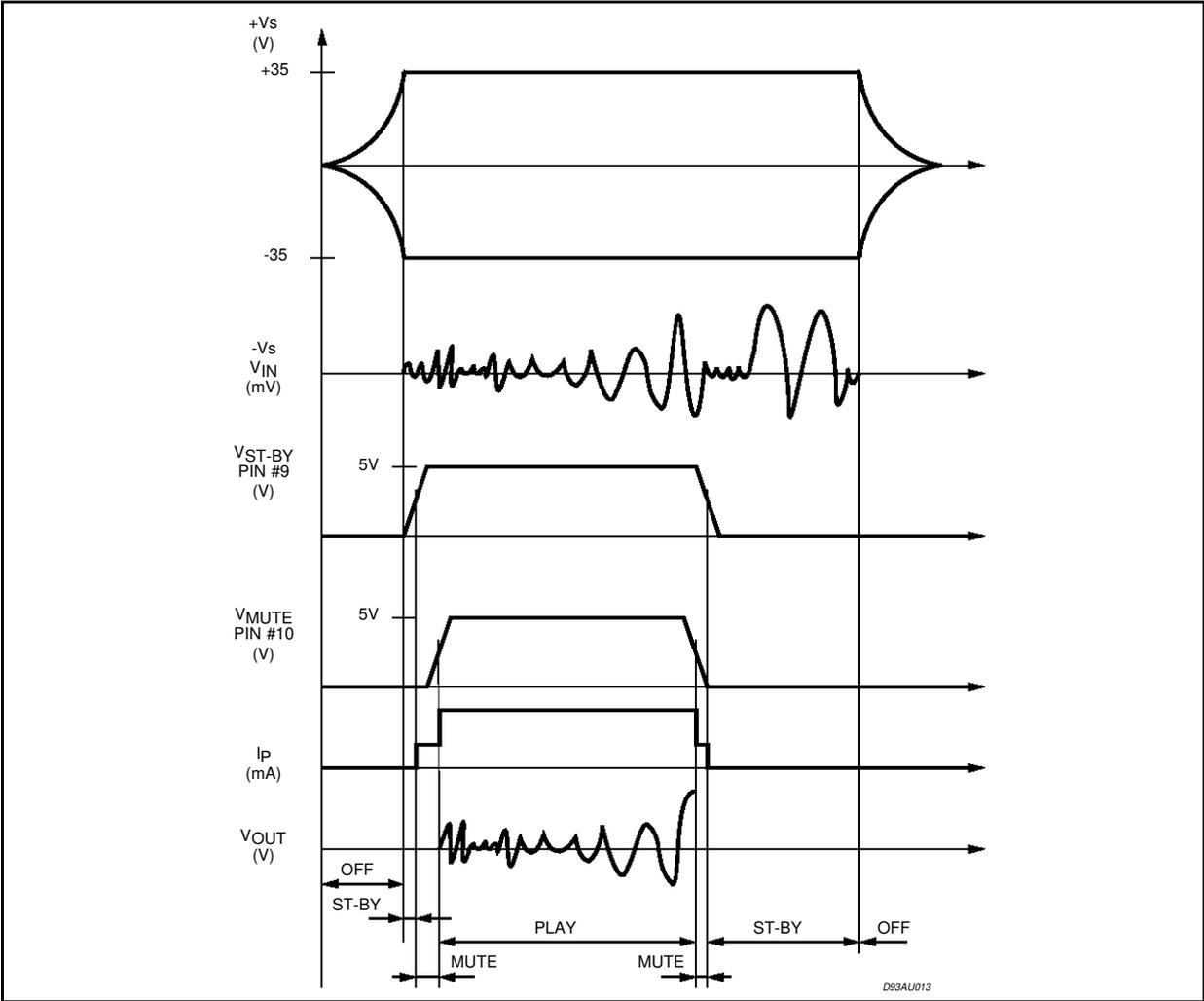
In addition to the overload protection described above, the device features a thermal shutdown circuit which initially puts the device into a muting state (@  $T_j = 145\text{ }^\circ\text{C}$ ) and then into stand-by (@
