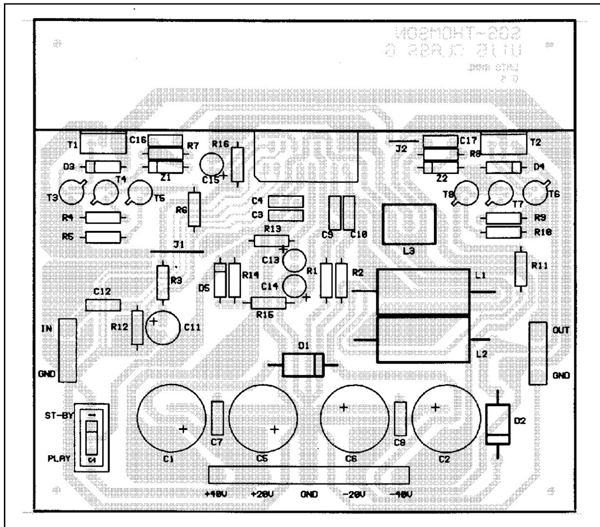
diodes Z1, Z2 and resistors R7, R8 define the minimum drop across the power MOS transistors of the TDA7294. L1, L2, L3 and the snubbers C9, R1 and C10, R2 stabilize the loops formed by the "bootstrap" circuits and the output stage of the TDA7294.
