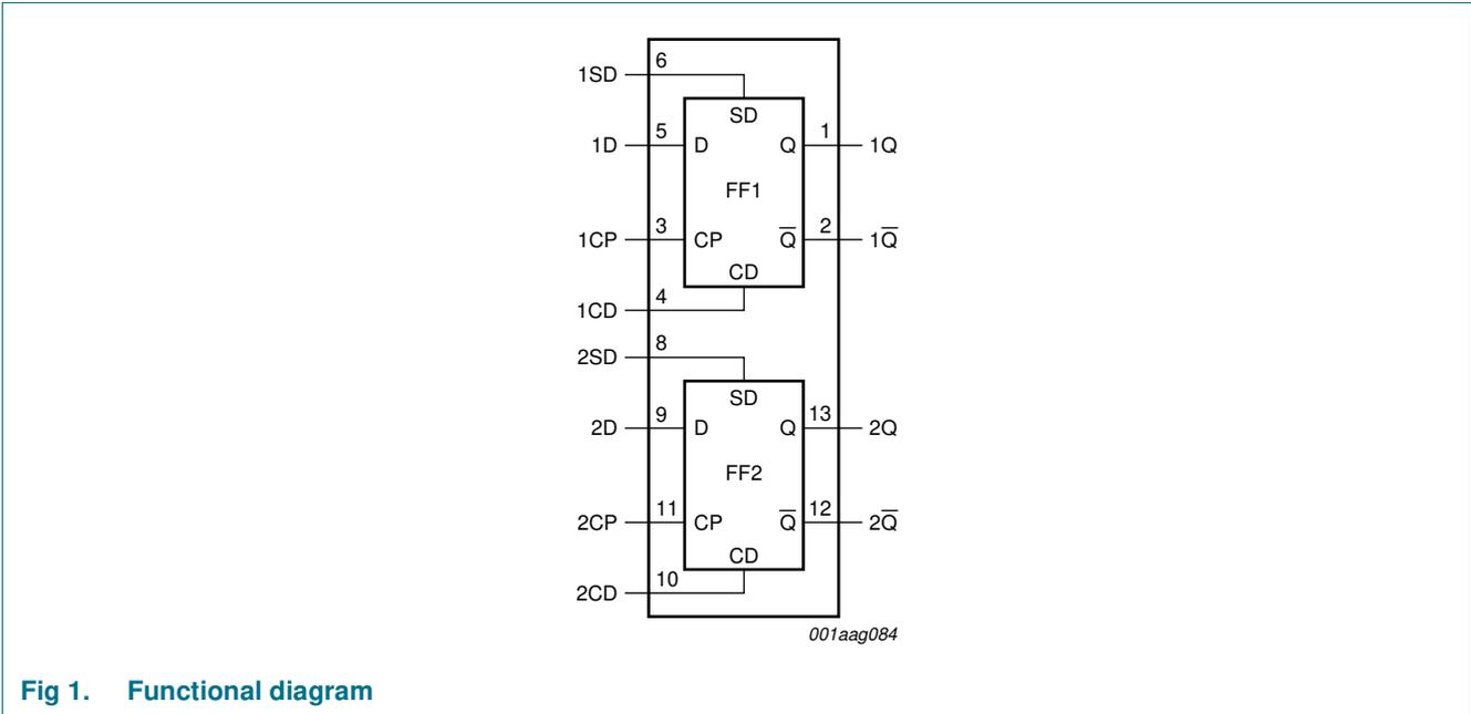
Fig 1. Functional diagram
