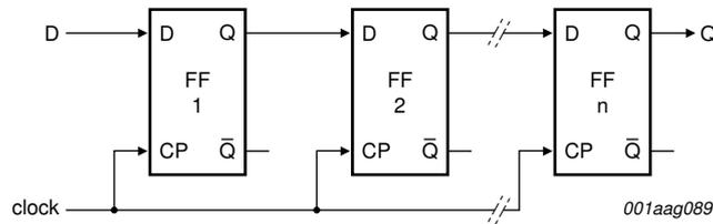
Fig 7. N-stage shift register
