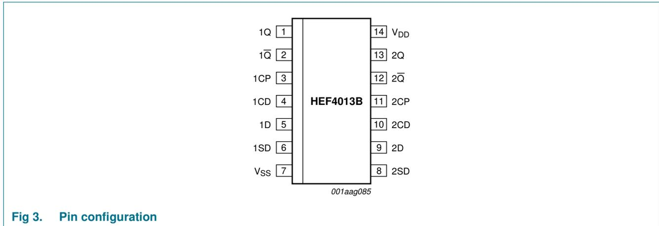
Fig 3. Pin configuration
