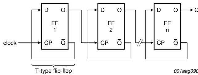
Fig 8. Binary ripple up-counter; divide-by-2<sup>n</sup>
