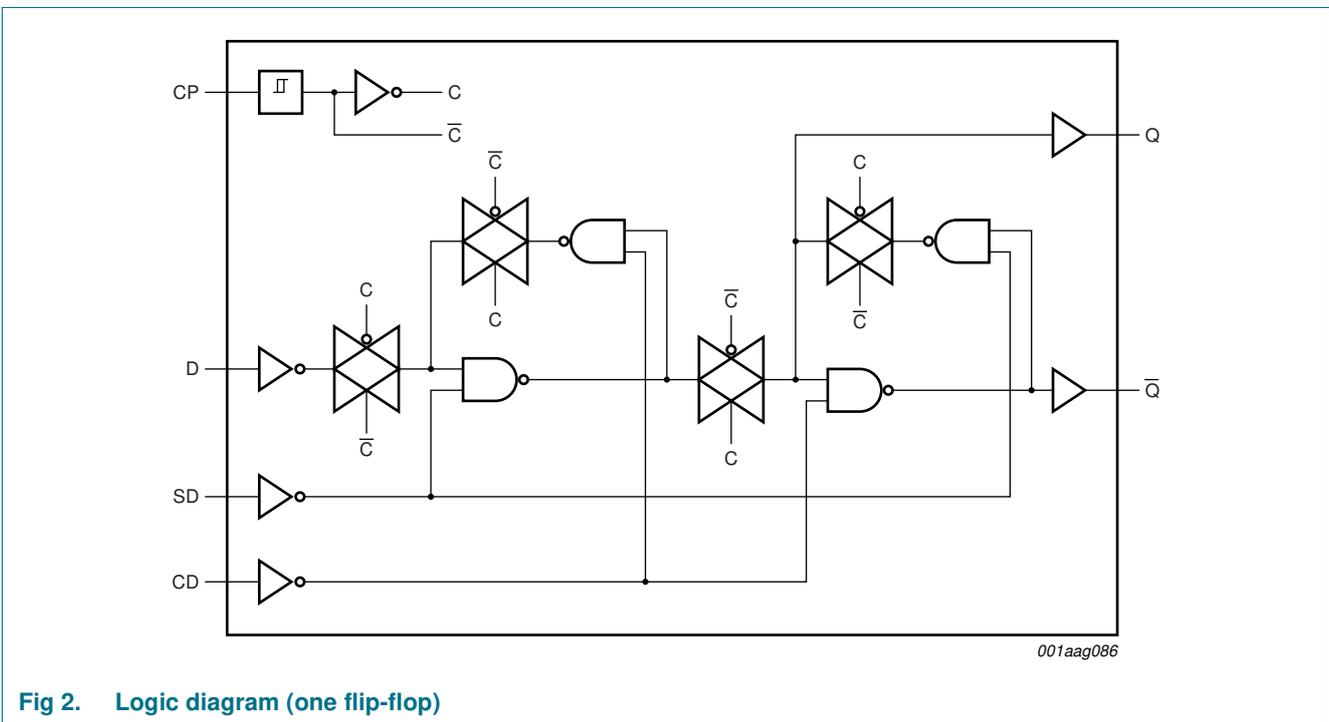
Fig 2. Logic diagram (one flip-flop)
