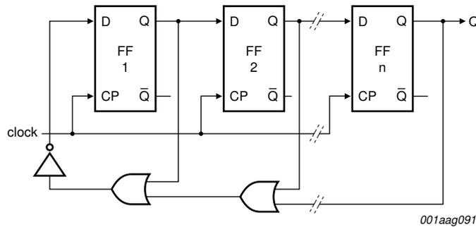
Fig 9. Modified ring counter; divide-by-(n + 1)
