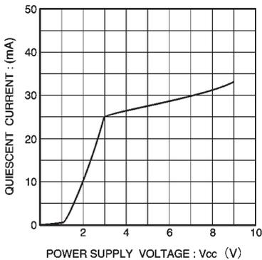
Fig. 4 Quiescent current vs. power supply voltage
