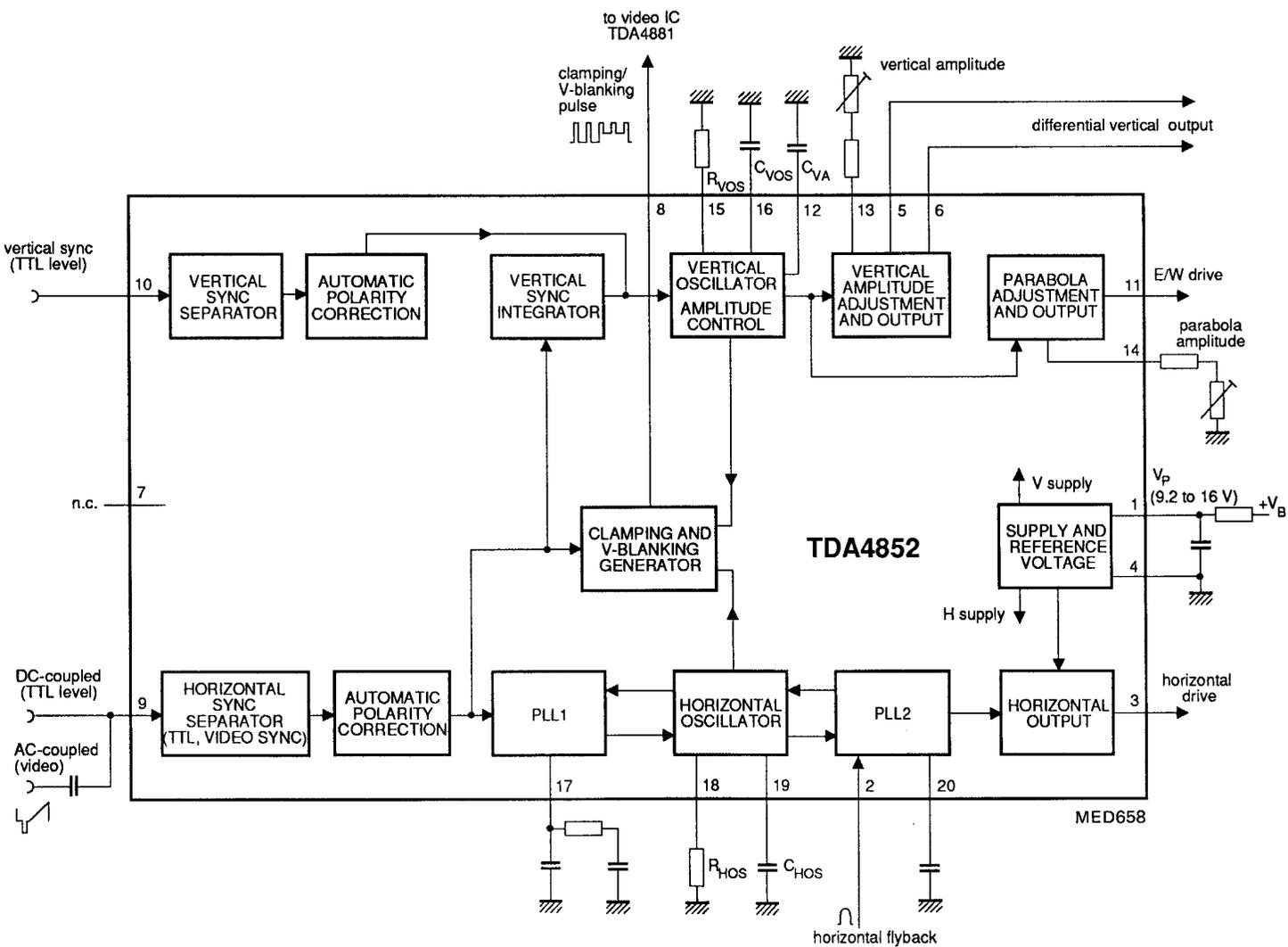
Fig.1 Block diagram.
