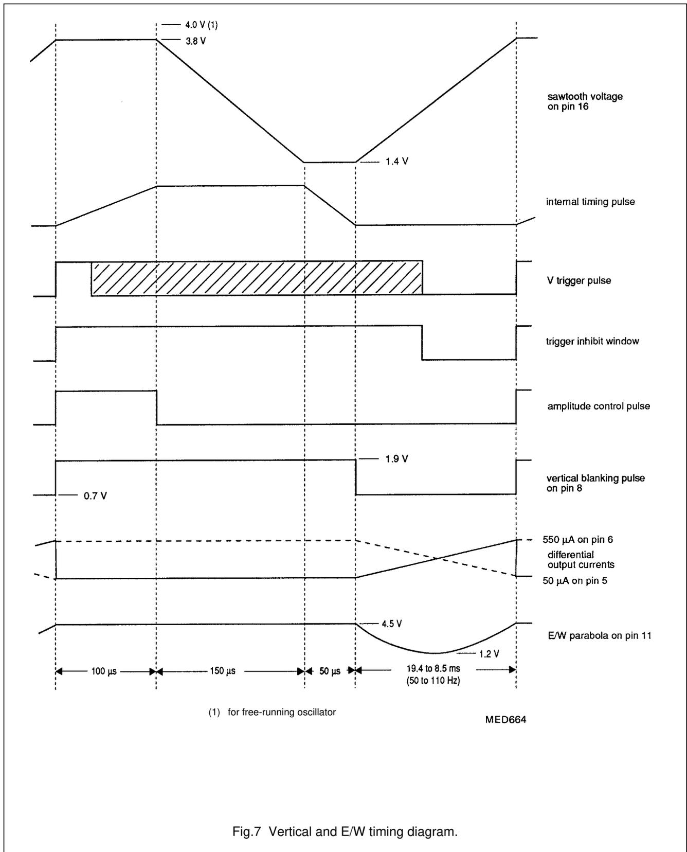
Fig.7 Vertical and E/W timing diagram.
