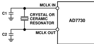
Figure 17. Crystal/Resonator Connections
