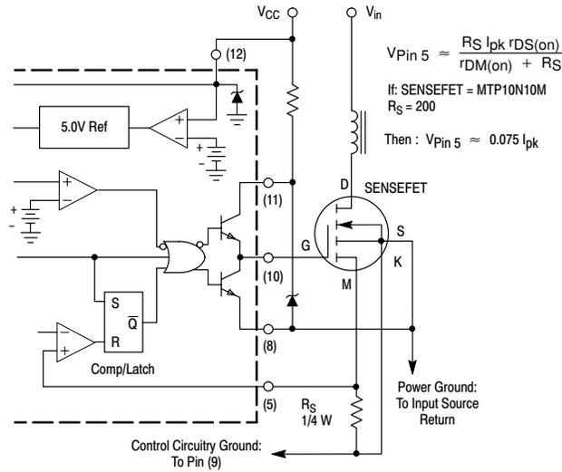
Virtually lossless current sensing can be achieved with the implementation of a SENSEFET power switch. For proper operation during over-current conditions, a reduction of the  $I_{pk(max)}$  clamp level must be implemented. Refer to Figures 23 and 25.
