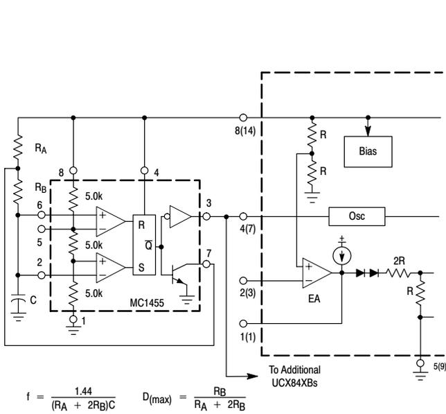
Figure 22. External Duty Cycle Clamp and Multi-Unit Synchronization
