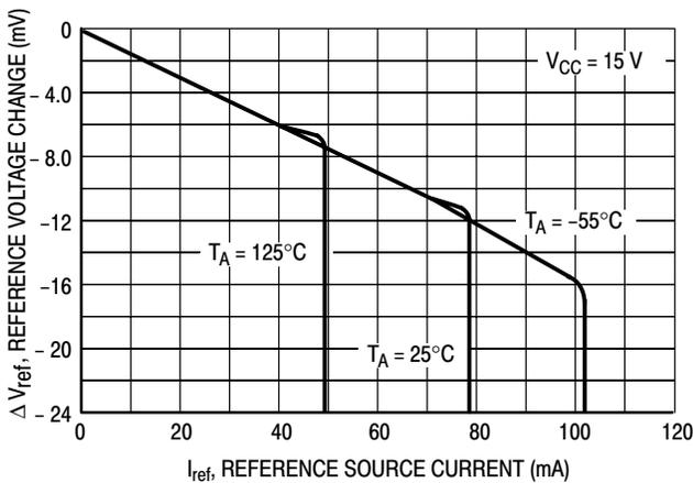
Figure 10. Reference Voltage Change versus Source Current
