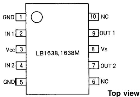
Note: both ground pins must be grounded.
