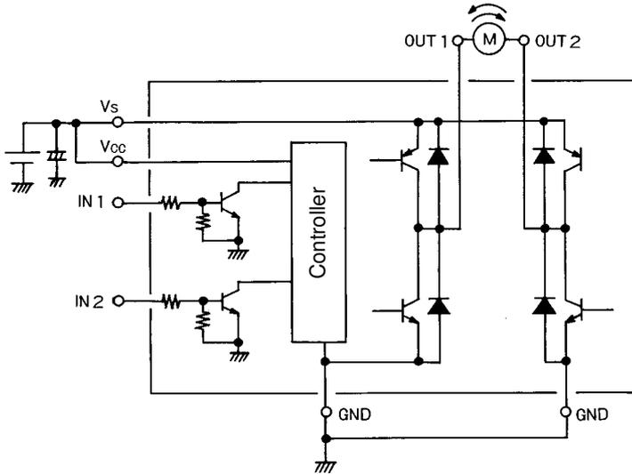
Note: When using the same power supply for  $V_S$  and  $V_{CC}$ , short the  $V_{CC}$  and  $V_S$  pins to each other or insert a capacitor in the  $V_{CC}$  line.
