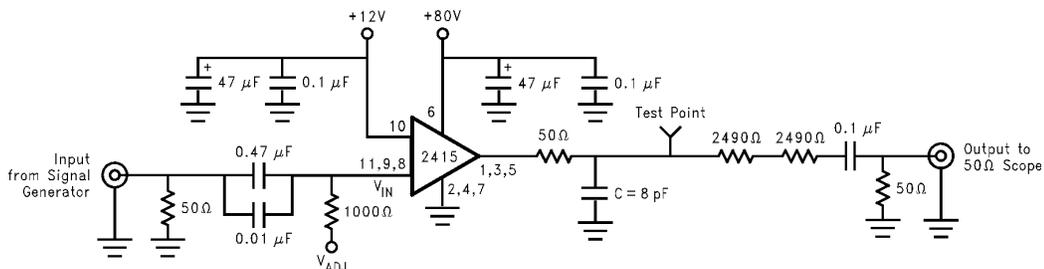
**Note:** 8 pF load includes parasitic capacitance.
