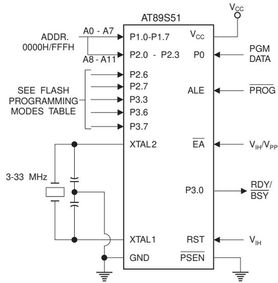
**Figure 5. Verifying the Flash Memory (Parallel Mode)**
