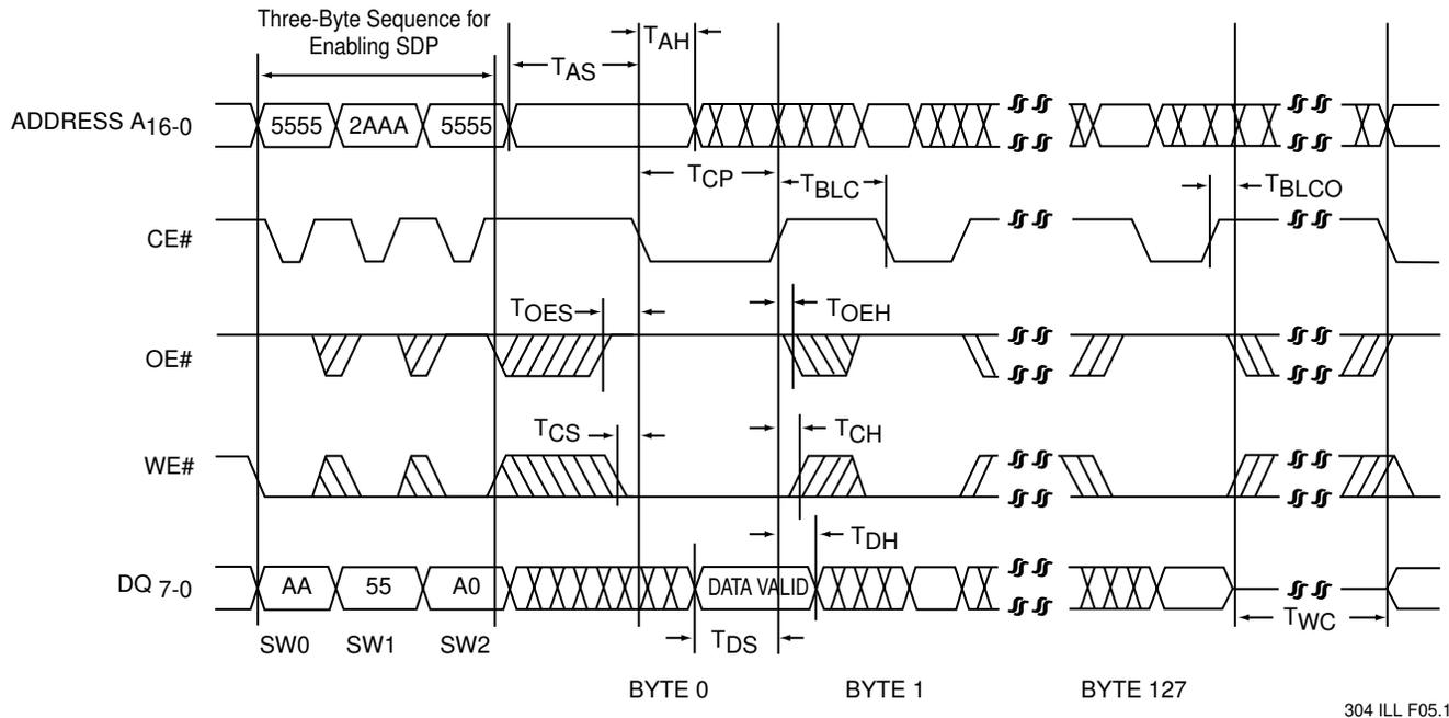
FIGURE 6: CE# CONTROLLED PAGE-WRITE CYCLE TIMING DIAGRAM
