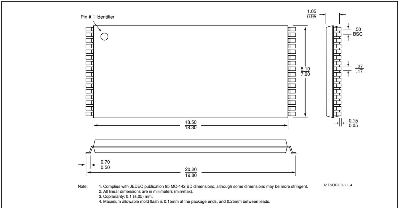
**32-LEAD THIN SMALL OUTLINE PACKAGE (TSOP) 8MM X 20MM**
