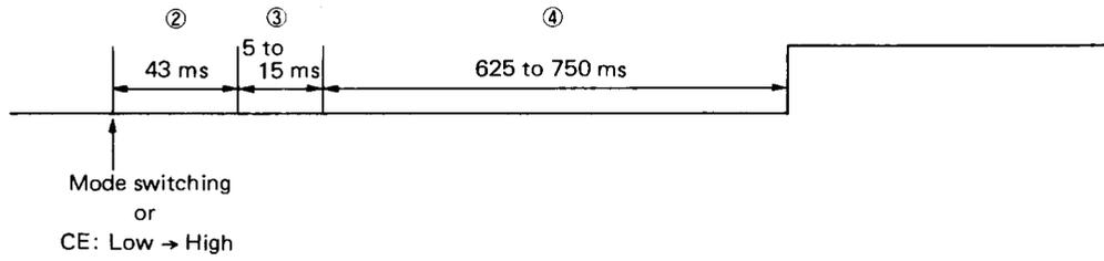
**(7) Mode switching (radio ON→OFF), CE pin: High→Low**
