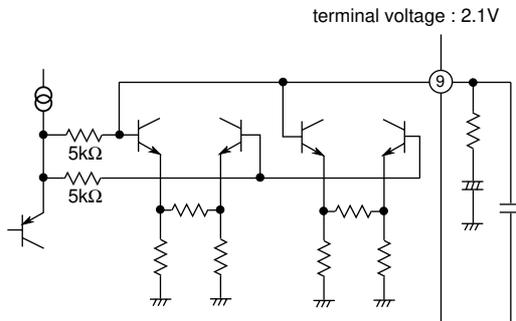
The FM detector can respond to several kinds of SIF signals without an adjustment and external components by adopting the PLL technique. It also is in compliance with the multi-SIF by selecting an appropriate deemphasis and audio output amplifier using the pin12 switch. The capacitor between pin 9 and 10, which fixes the deemphasis characteristics, can be determined considering the combination of an equivalent resistance of the IC and this capacitor itself.
