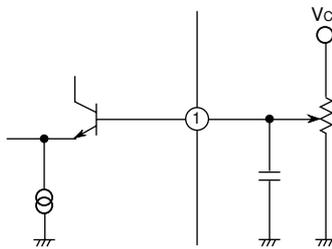
An applied voltage to the pin1 is for changing a RF AGC delay point.
