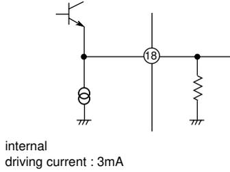
An output amplitude is positive 2Vp-p in the case of 87.5% video modulation.
