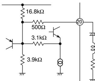
Both the external coil and capacitor determine the frequency response of EQ output. The series connected resistor is for damping.
