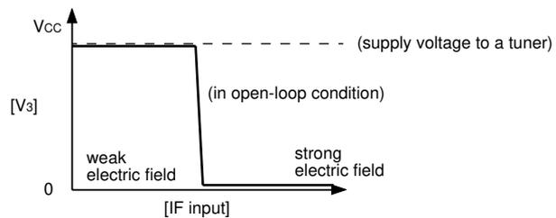
Note: Connecting a nonpolarity capacitor of 1μF between pin1 and pin 3 improves AGC operating speed.
