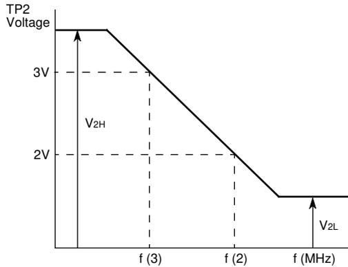
$$\mu = \frac{1000 \text{ (mV)}}{f(2) - f(3) \text{ (kHz)}} \text{ (mV/kHz)}$$
