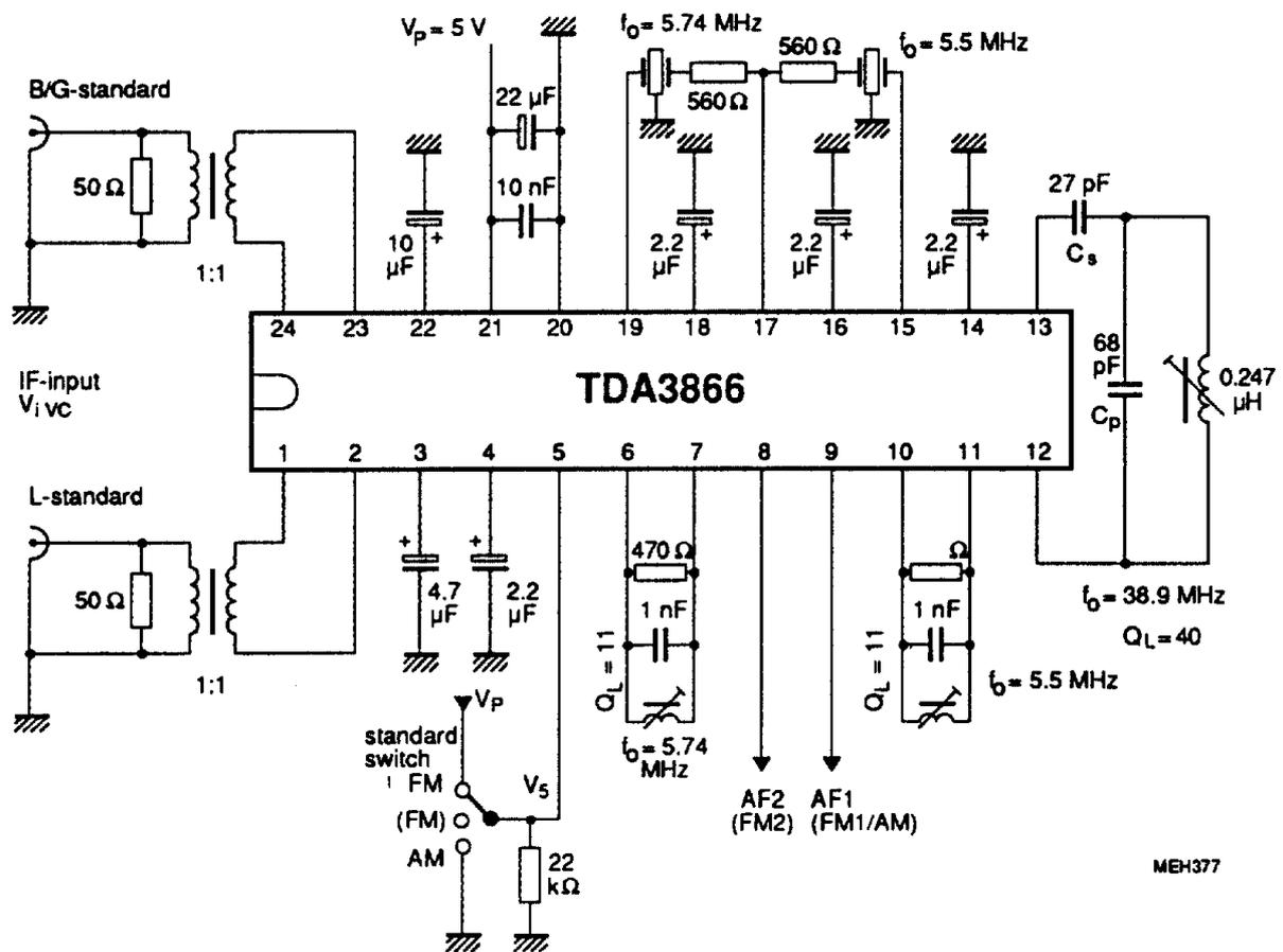
Fig.3 Test and application circuit for standards B/G and L (for application SAW-filters must be used).
