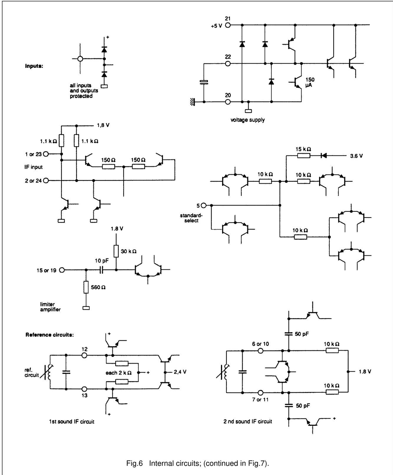
Fig.6 Internal circuits; (continued in Fig.7).
