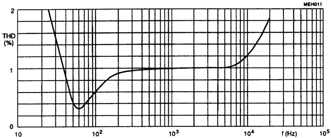
Fig.4 Total harmonic distortion (THD) as a function of audio frequency at AM standard ( $V_5 = 0$ ).
