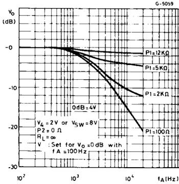
**Figure 4 :** Amplitude Modulation Rejection vs. Input Signal.
