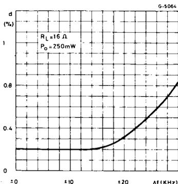
**Figure 9 :** Distortion vs. Tuning Frequency Change.
