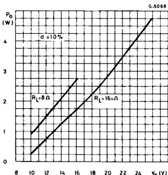
**Figure 13 :** Power Dissipation vs. Supply Voltage (sine Wave operation).
