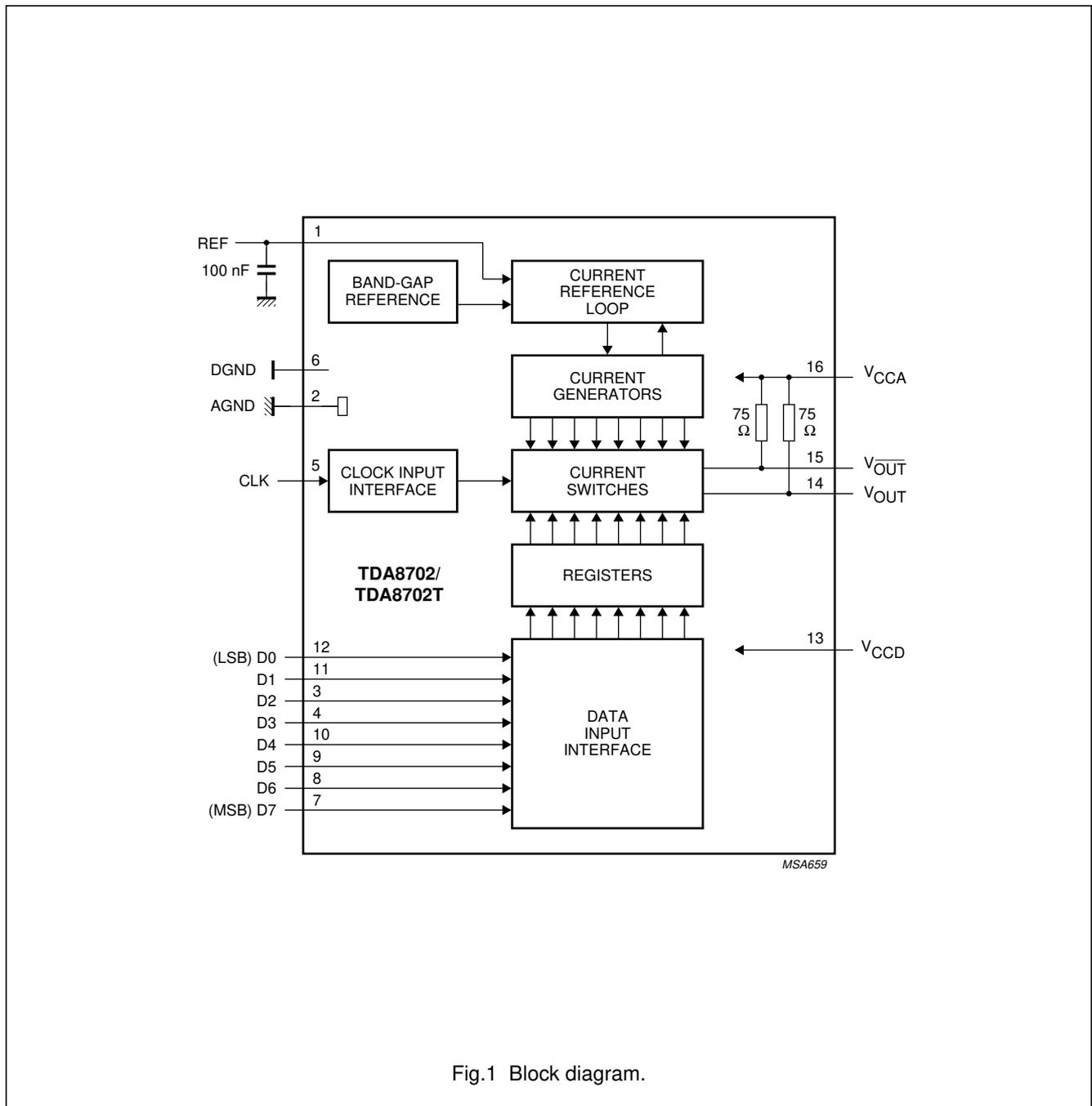
Fig.1 Block diagram.
