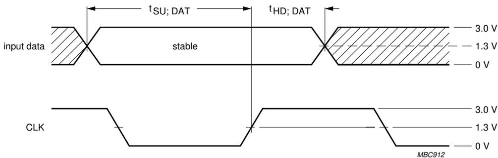
The shaded areas indicate when the input data may change and be correctly registered. Data input update must be completed within 0.3 ns after the first rising edge of the clock ( $t_{SU; DAT}$  is negative; -0.3 ns). Data must be held at least 2 ns after the rising edge ( $t_{HD; DAT} = +2$  ns).
