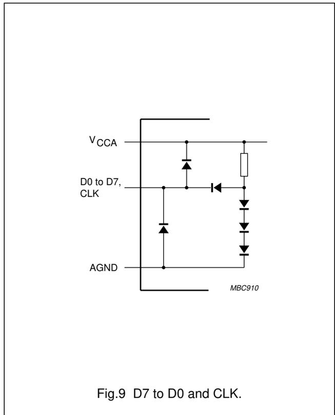
8-bit video digital-to-analog converter
