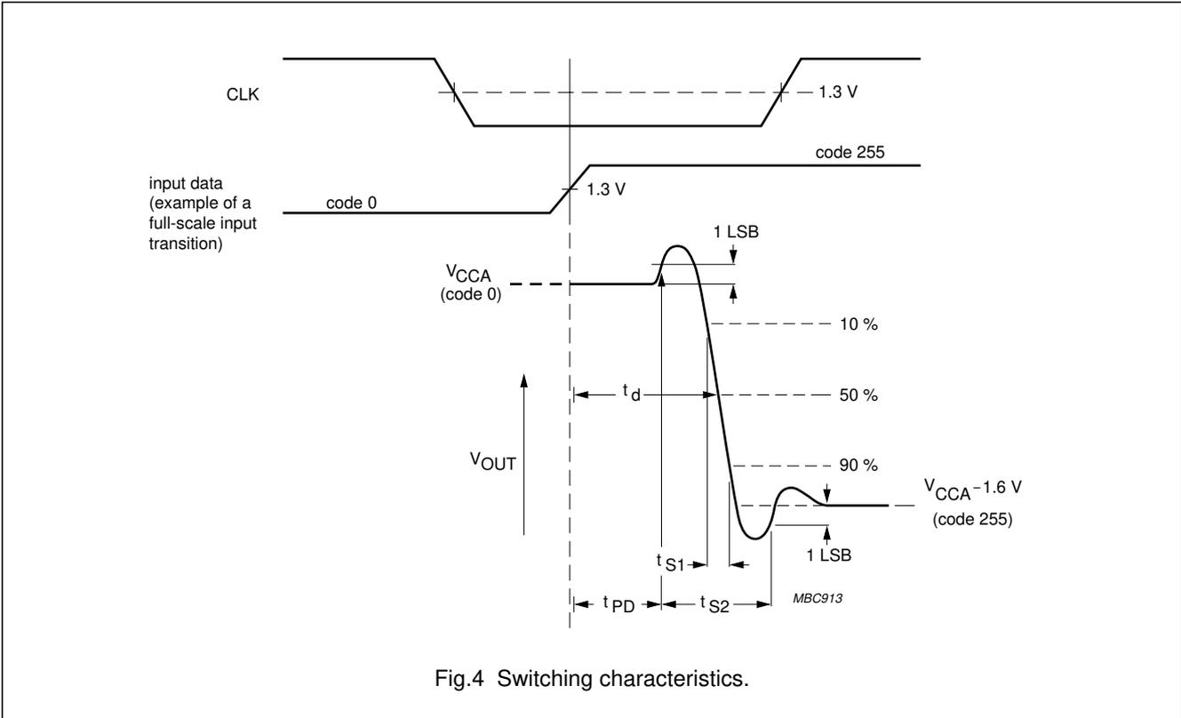
Fig.4 Switching characteristics.
