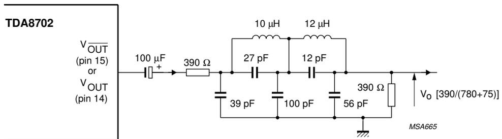
Fig.16 Example of anti-aliasing filter (analog output referenced to AGND).
