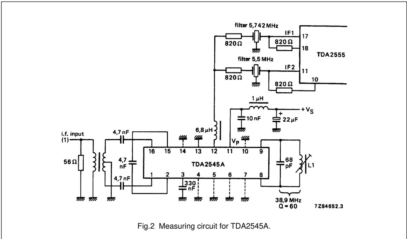
Fig.2 Measuring circuit for TDA2545A.
