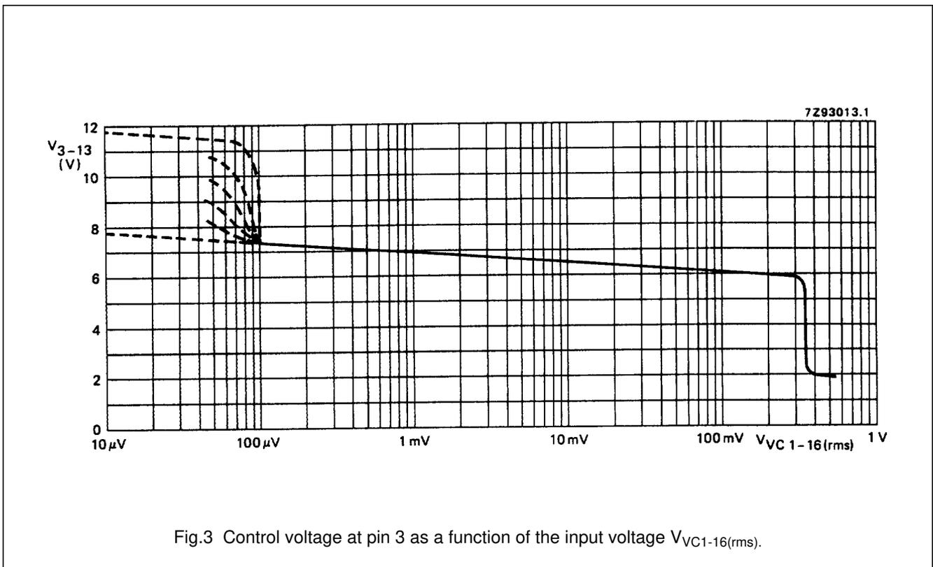
Fig.3 Control voltage at pin 3 as a function of the input voltage  $V_{VC1-16(rms)}$ .
