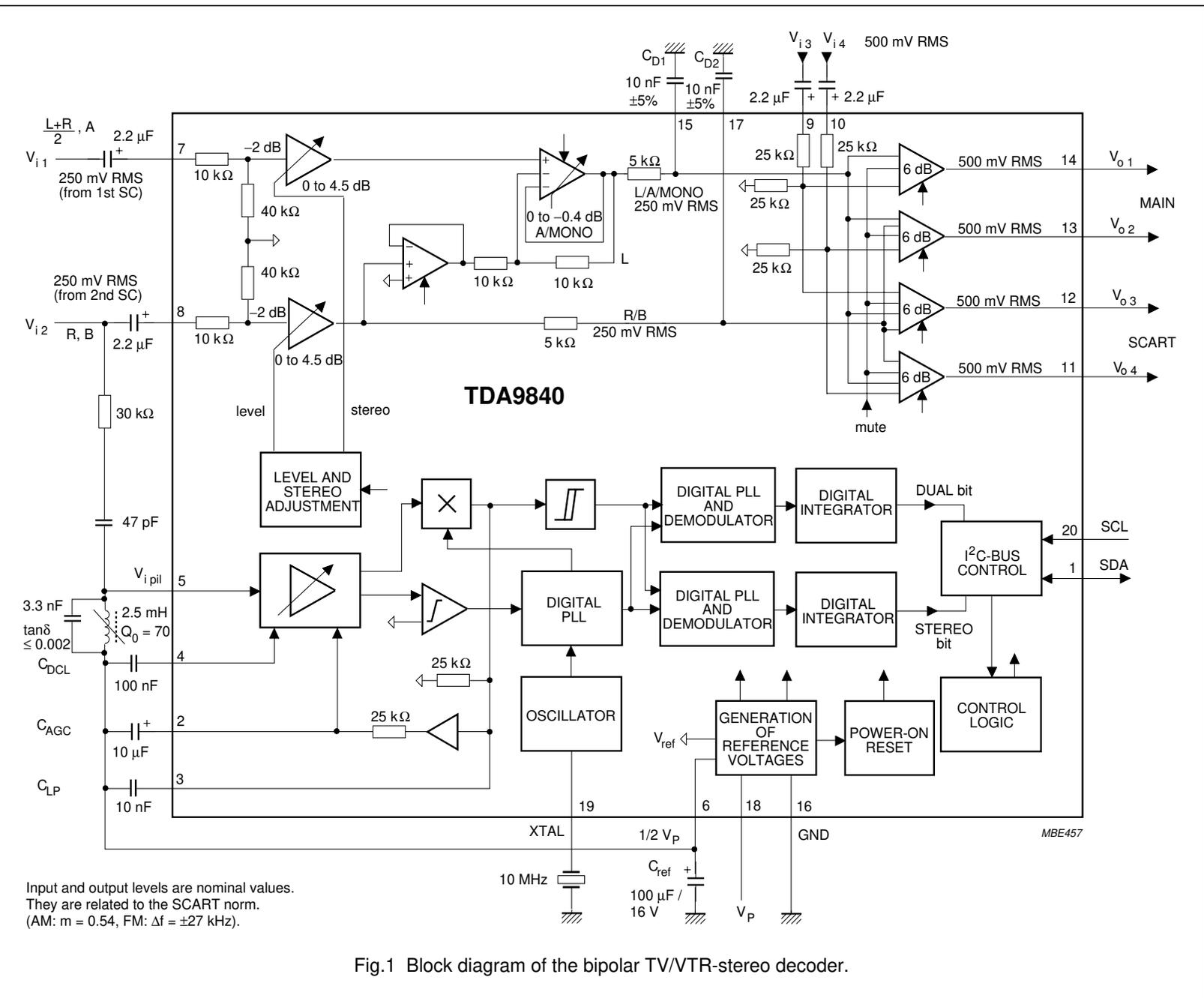
Fig.1 Block diagram of the bipolar TV/VTR-stereo decoder.
