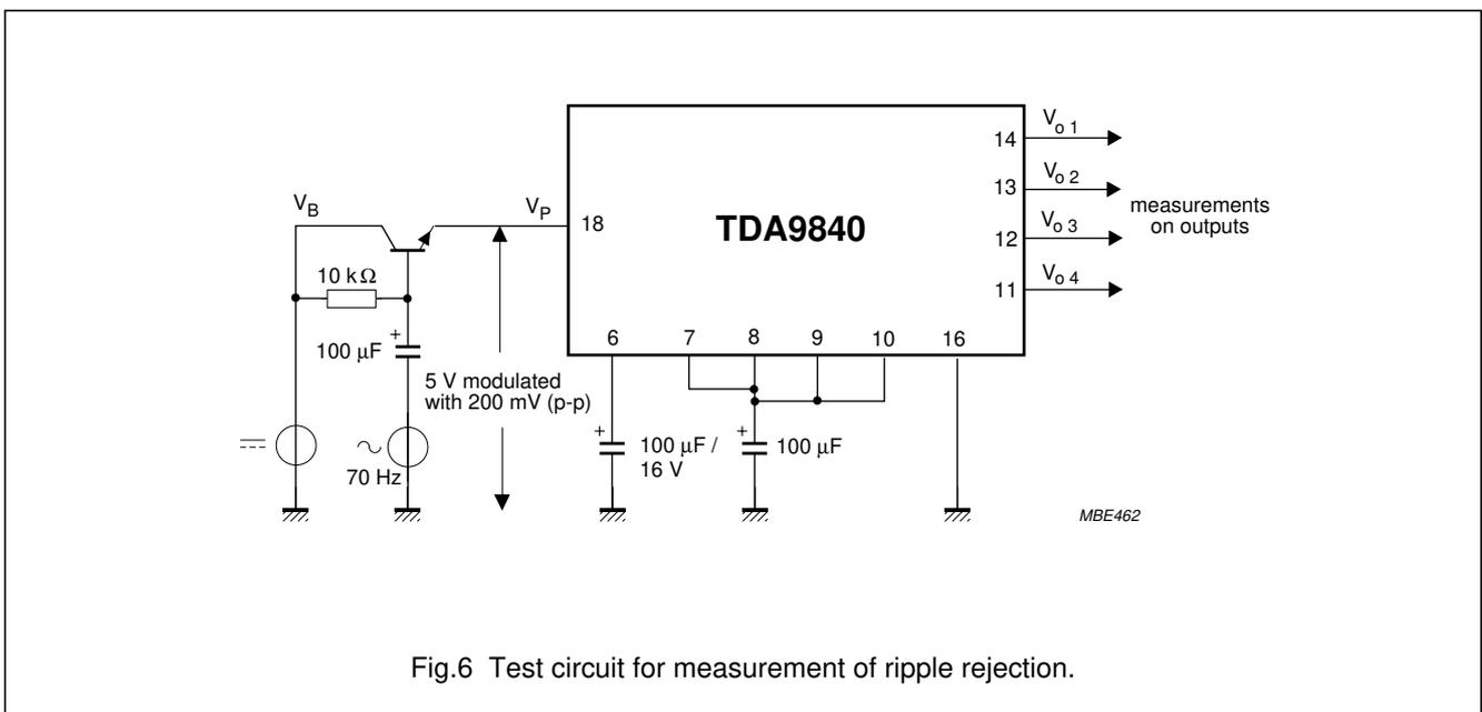
Fig.6 Test circuit for measurement of ripple rejection.
