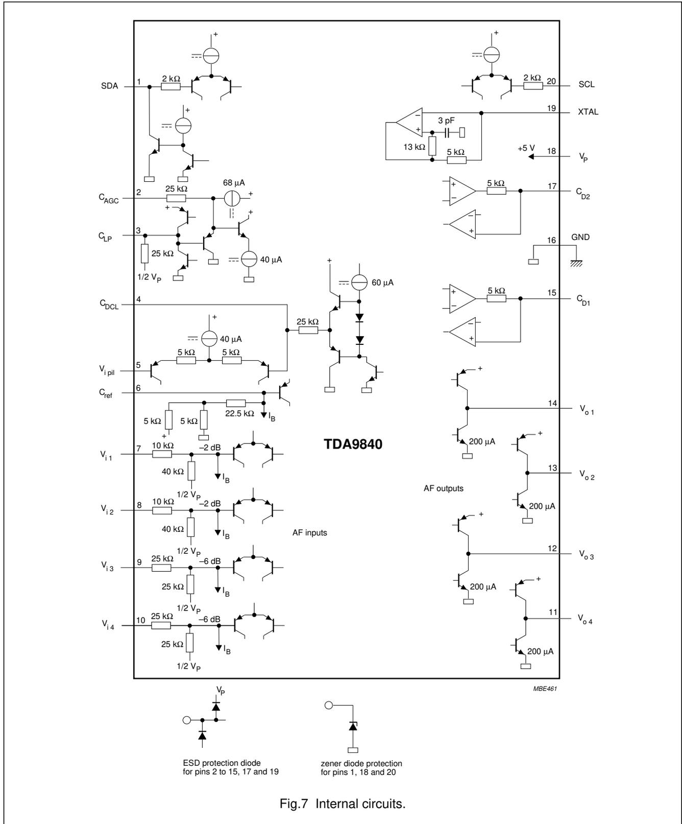
Fig.7 Internal circuits.
