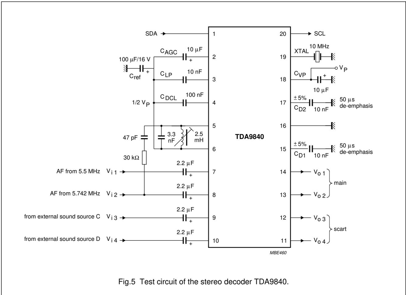
Fig.5 Test circuit of the stereo decoder TDA9840.
