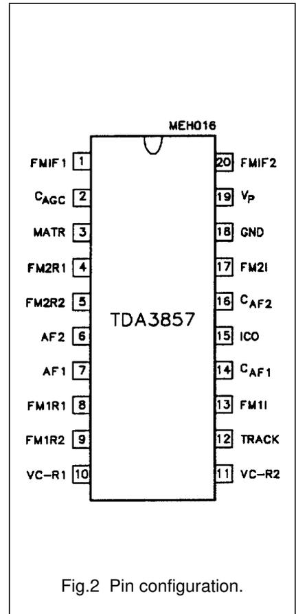
Fig.2 Pin configuration.
