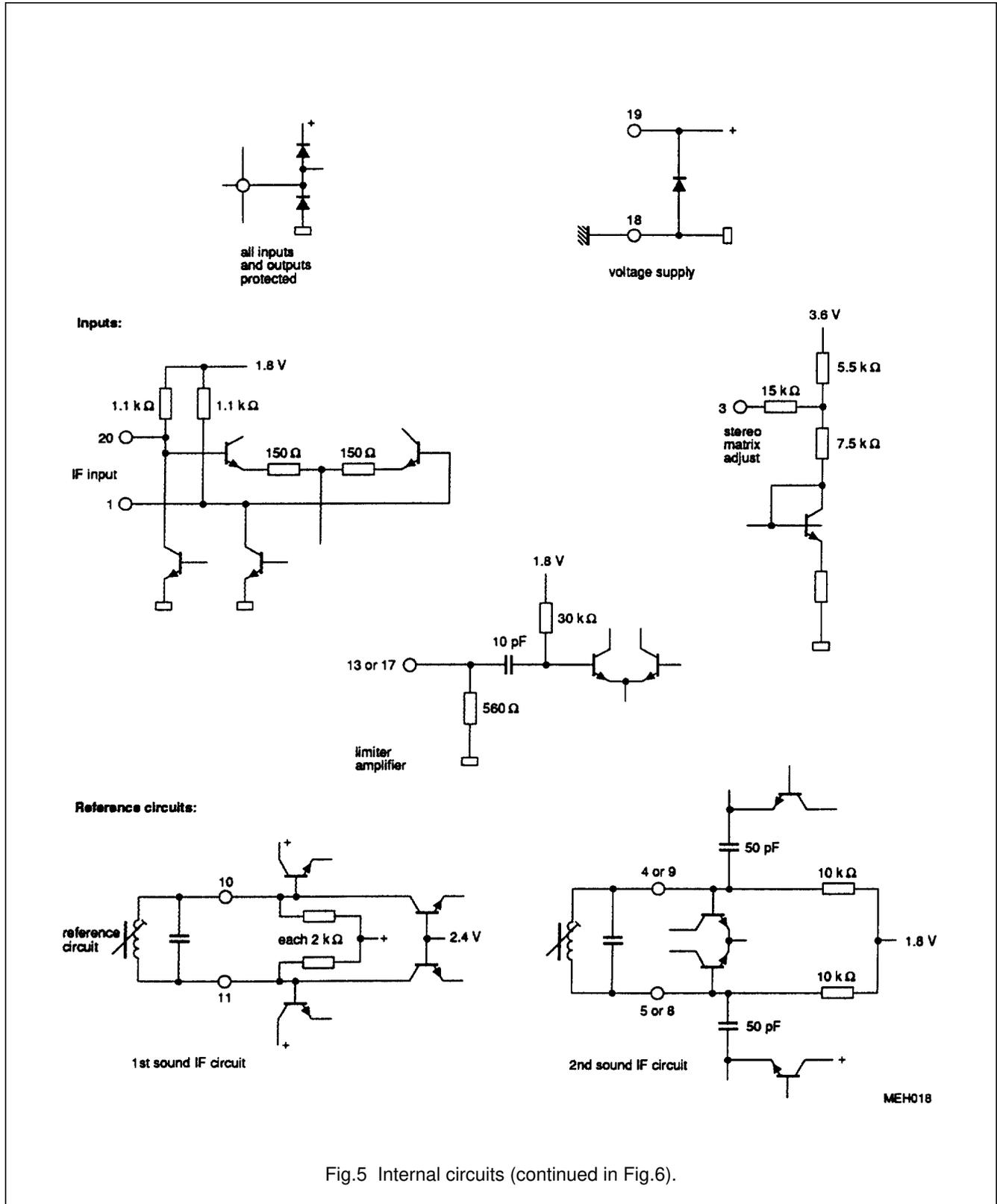
Fig.5 Internal circuits (continued in Fig.6).
