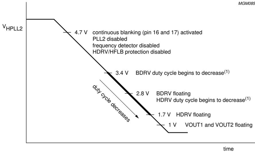
b. PLL2 soft-down sequence, via the I<sup>2</sup>C-bus, if V<sub>CC</sub> > 8.6 V.
