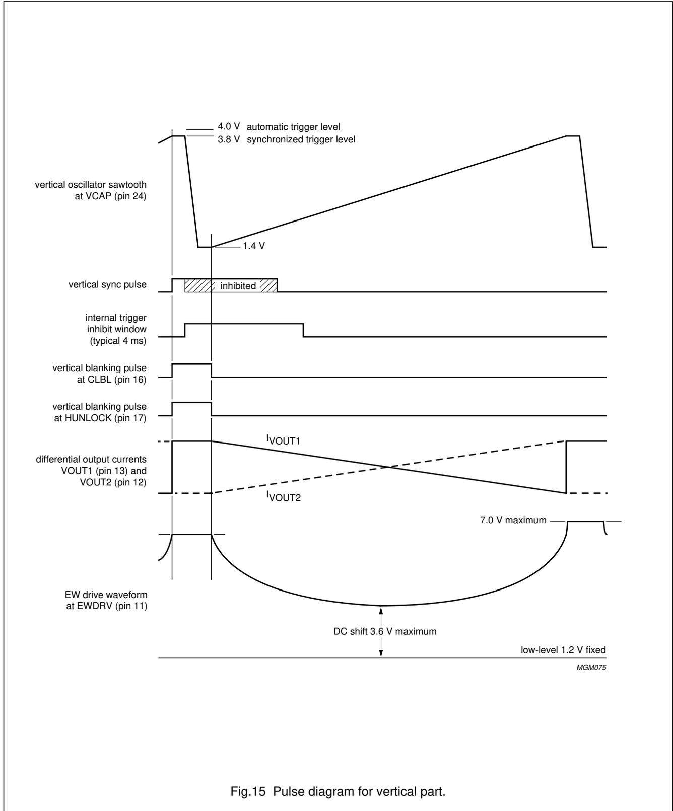
Fig.15 Pulse diagram for vertical part.
