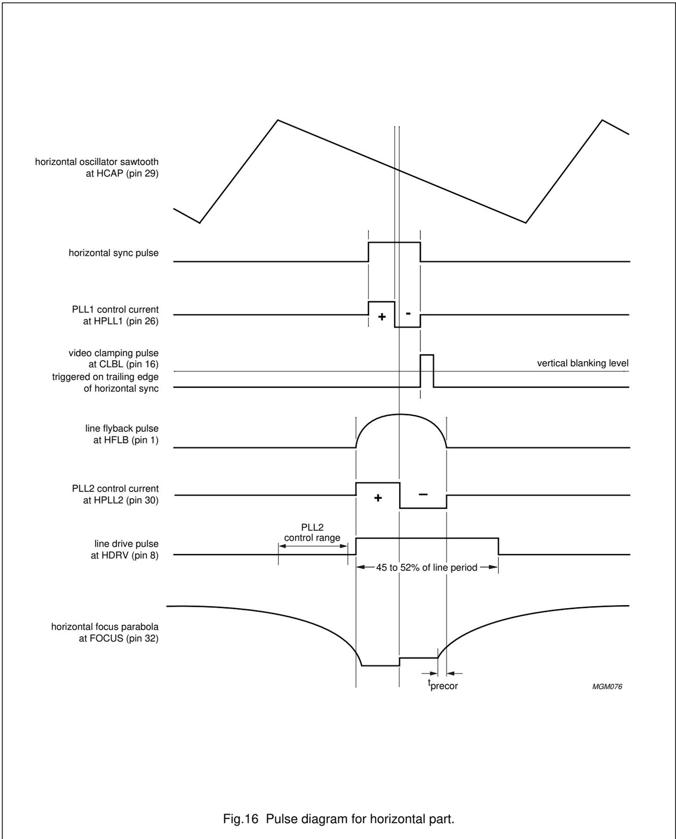
Fig.16 Pulse diagram for horizontal part.
