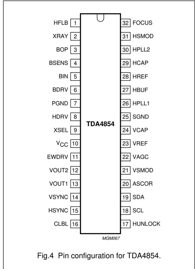
Fig.4 Pin configuration for TDA4854.
