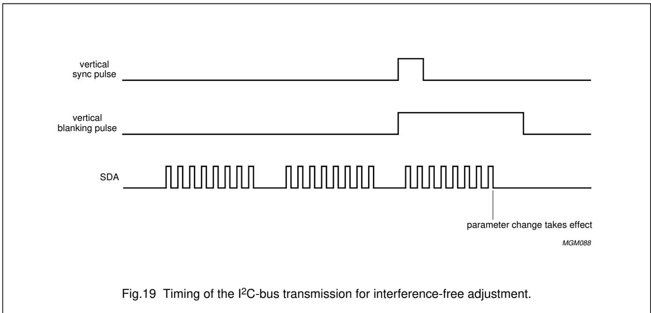
Fig.19 Timing of the I<sup>2</sup>C-bus transmission for interference-free adjustment.
