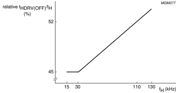
Fig. 17 Relative t<sub>OFF</sub> time of HDRV as a function of horizontal frequency.
