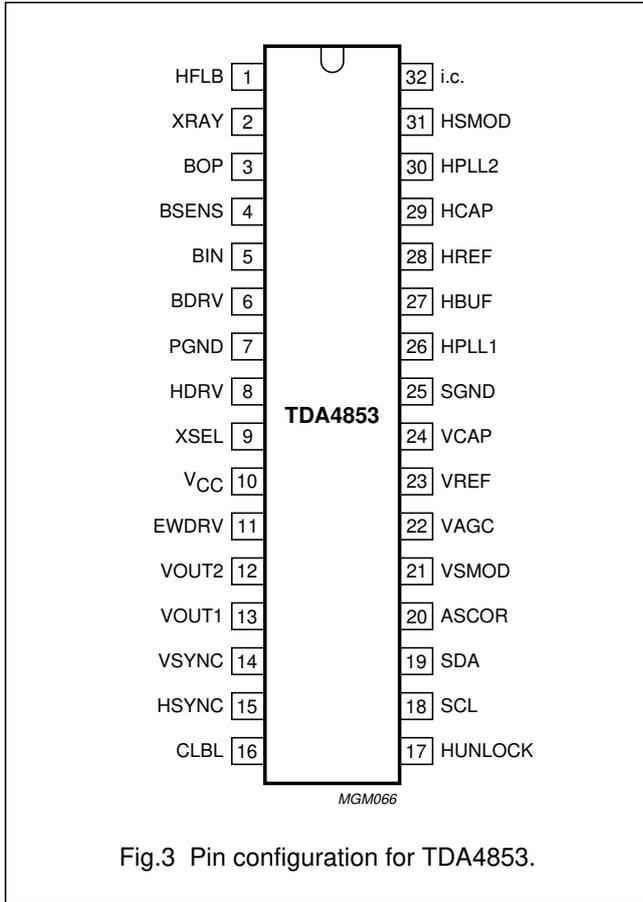
Fig.3 Pin configuration for TDA4853.
