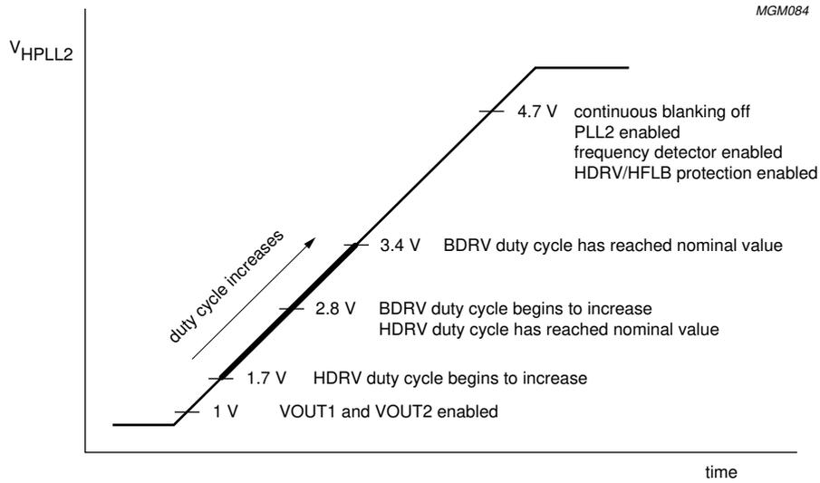
a. PLL2 soft start sequence, via the I<sup>2</sup>C-bus, if V<sub>CC</sub> > 8.6 V.
