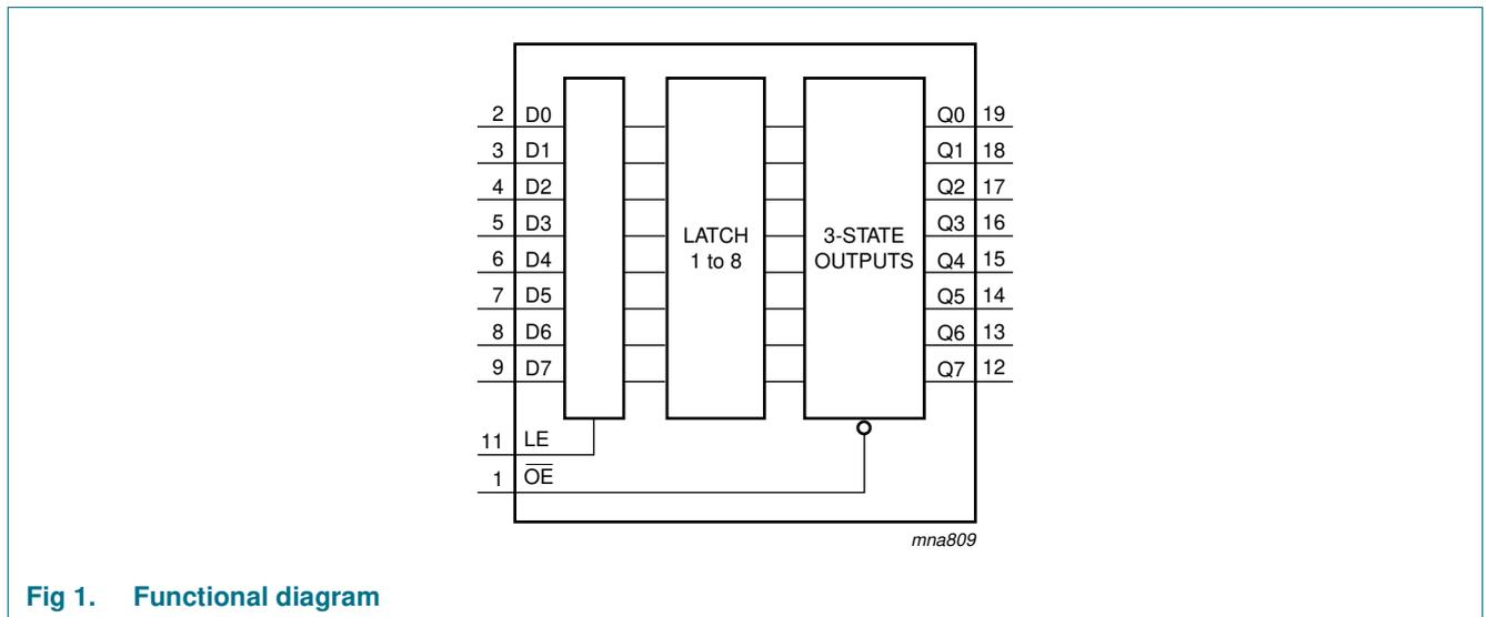
Fig 1. Functional diagram
