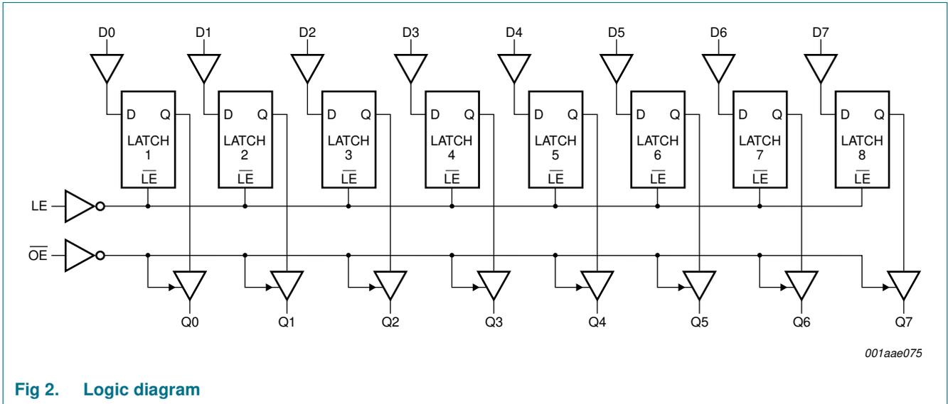
Fig 2. Logic diagram
