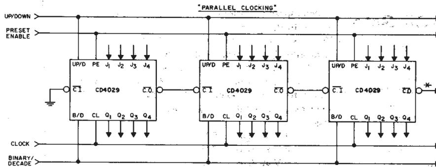
\* CARRY OUT lines at the 2nd, 3rd, etc., stages may have a negative-going glitch pulse resulting from differential delays of different CD4029B IC's. These negative-going glitches do not affect proper CD4029B operation. However, if the CARRY OUT signals are used to trigger other edge-sensitive logic devices, such as FF's or counters, the CARRY OUT signals should be gated with the clock signal using a 2-input OR gate such as CD4071B.
