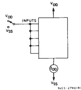
Fig. 14 – Quiescent device current test circuit.
