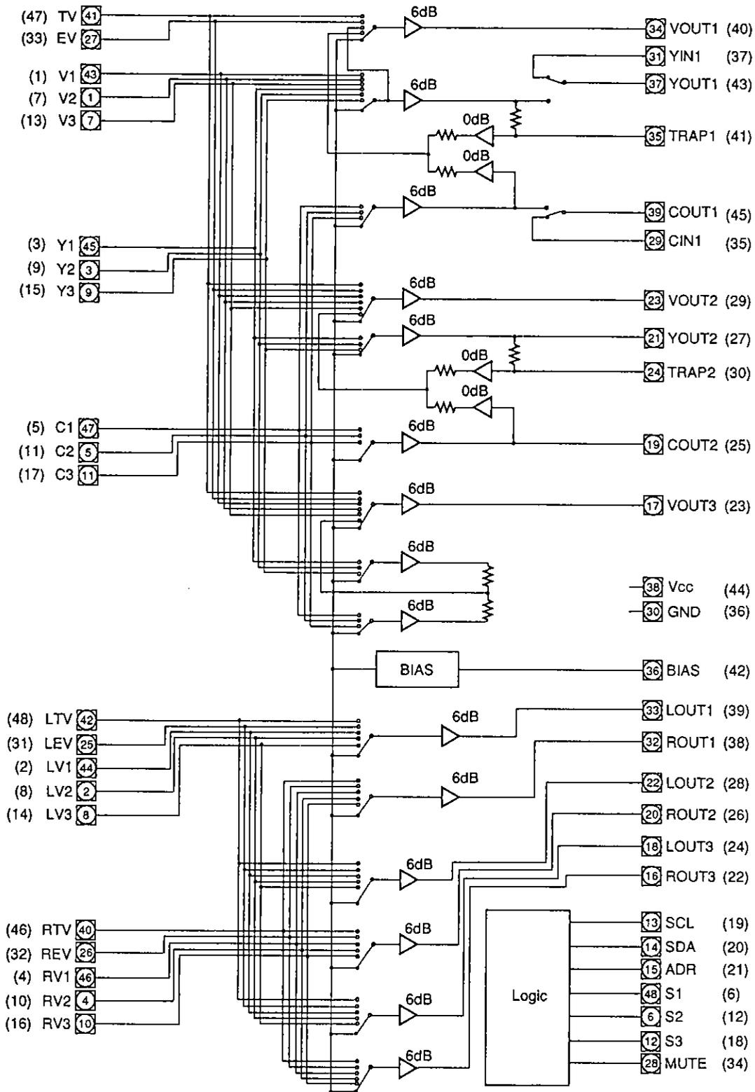
**Note)** A total gain of 0dB is achieved by connecting a 6kΩ resistor to the each audio input.
